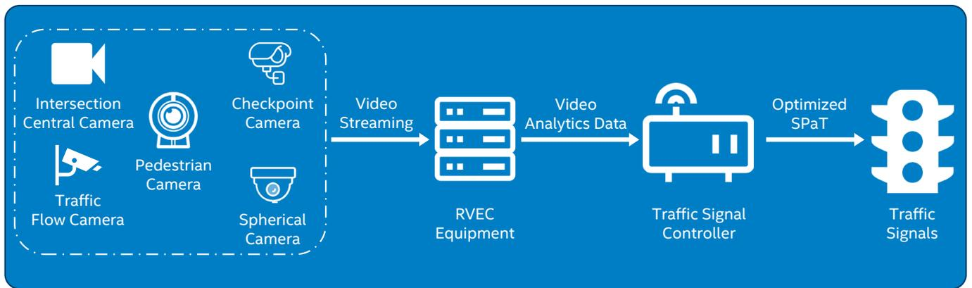
Figure 4. RVEC equipment for automatic traffic signal control.
