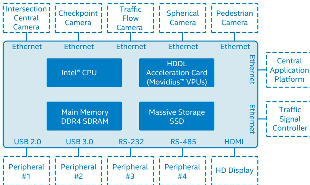
Figure 2. Hardware architecture of RVEC equipment.
