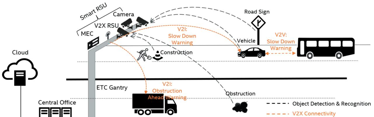
Figure 6. Vehicle-Infrastructure Integration (VII) based on MEC and C-V2X.
