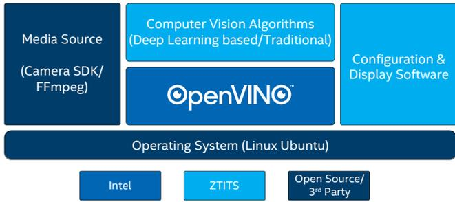
Figure 3. Software architecture of RVEC equipment.
