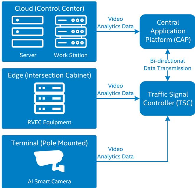
Figure 1. ITMS based on the "Terminal-Edge-Cloud" architecture.
