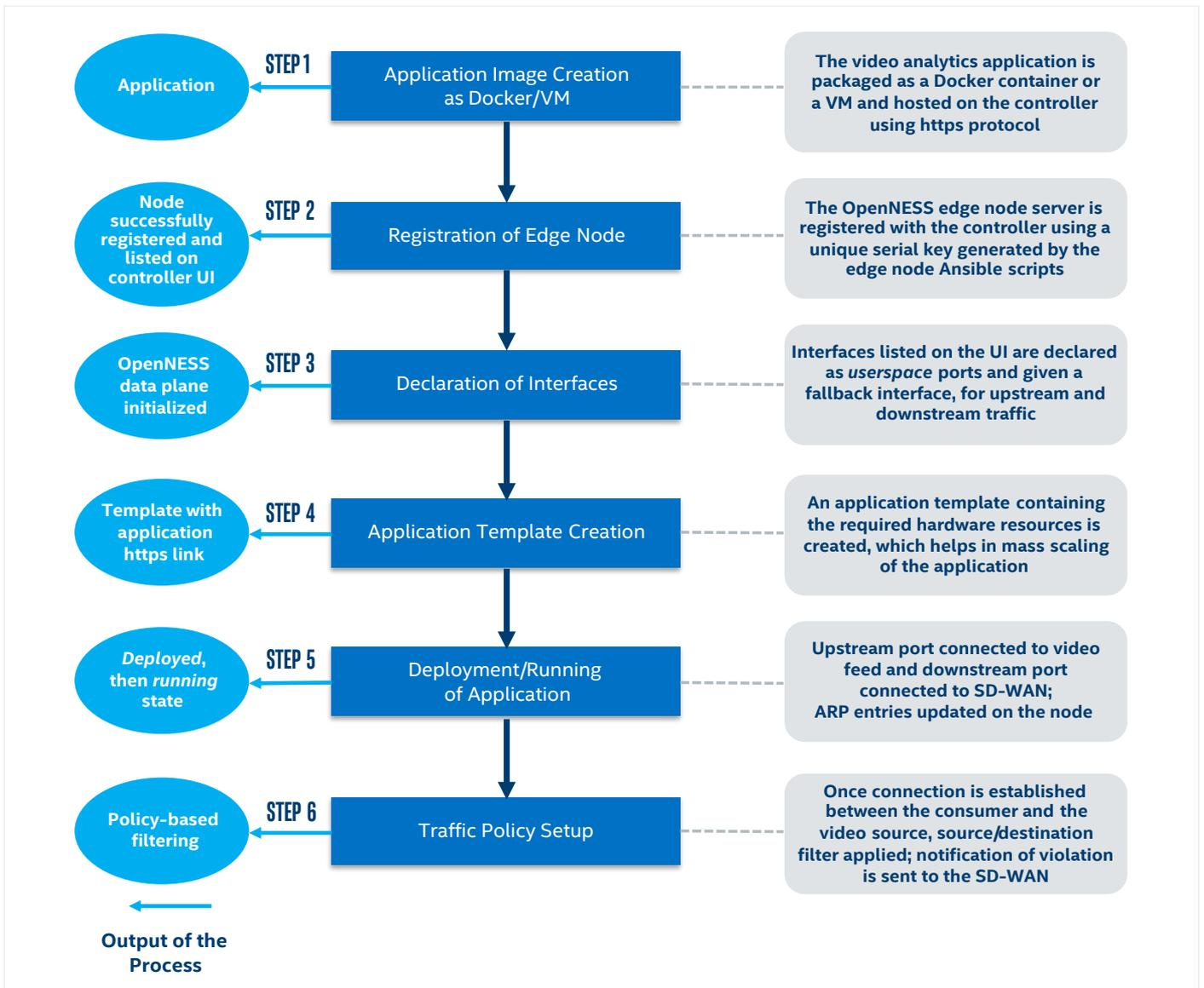
Figure 5. Flow diagram for application deployment on edge.
