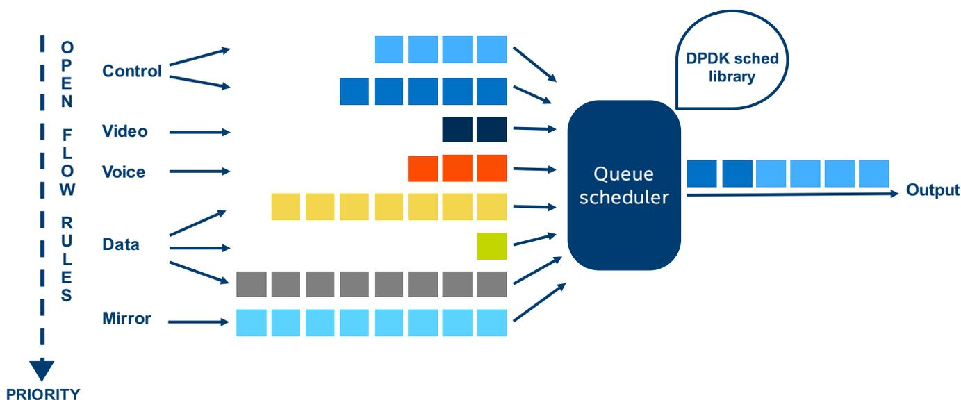
Figure 1. Priority queuing for Flow-based QoS for OVS with DPDK
