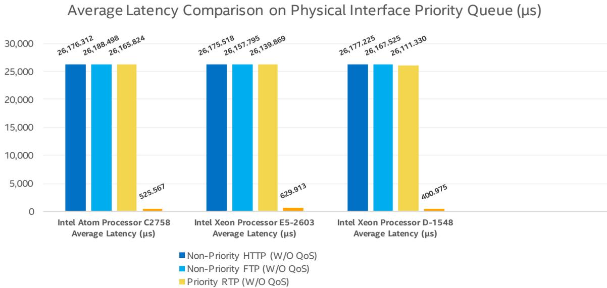
Figure 2. Average latency for QoS and non QoS testing in Intel and Wipro PoC<sup>1</sup>
