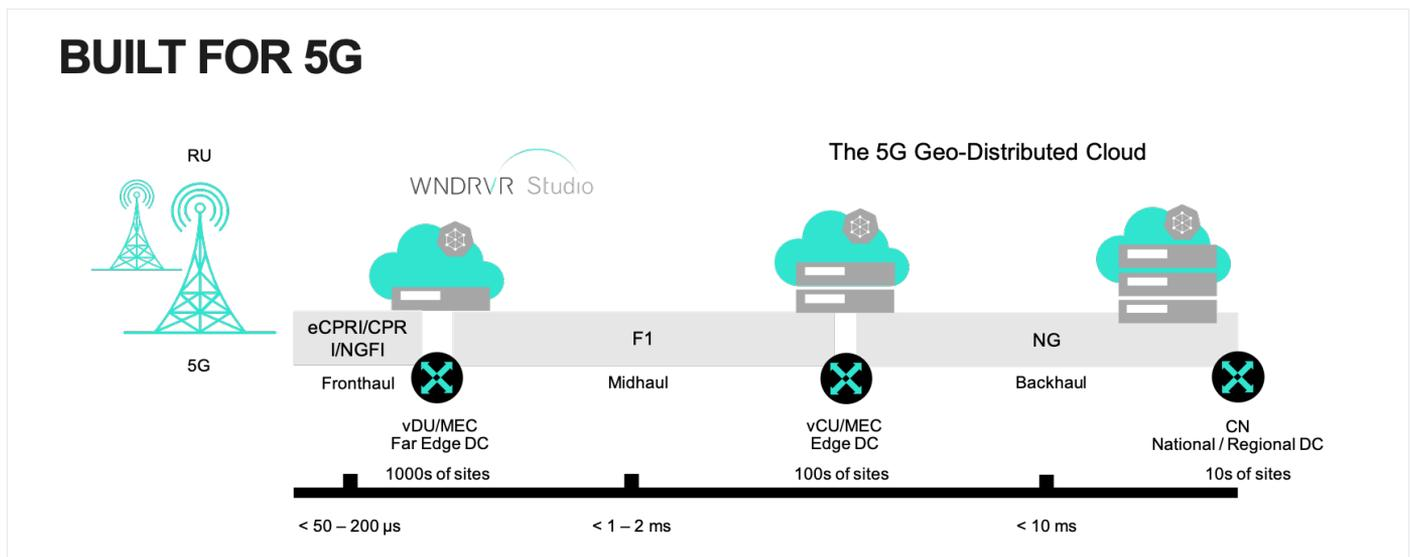
Figure 1. Wind River Cloud Platform deployed as a single geo-distributed cloud.
