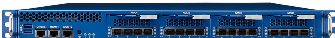
Figure 2. Advantech FWA-5020 configured as a Casa Systems Security Gateway
