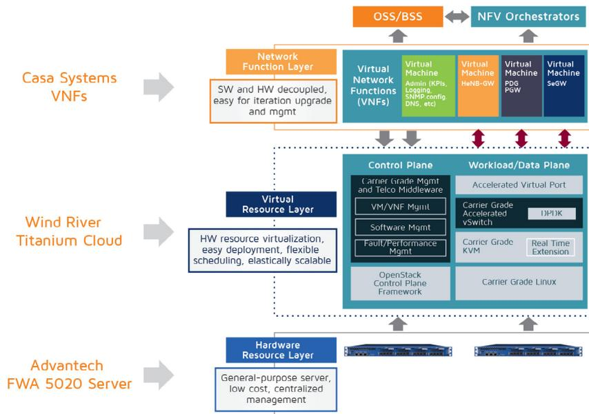
Figure 1. Virtual security gateway system architecture
