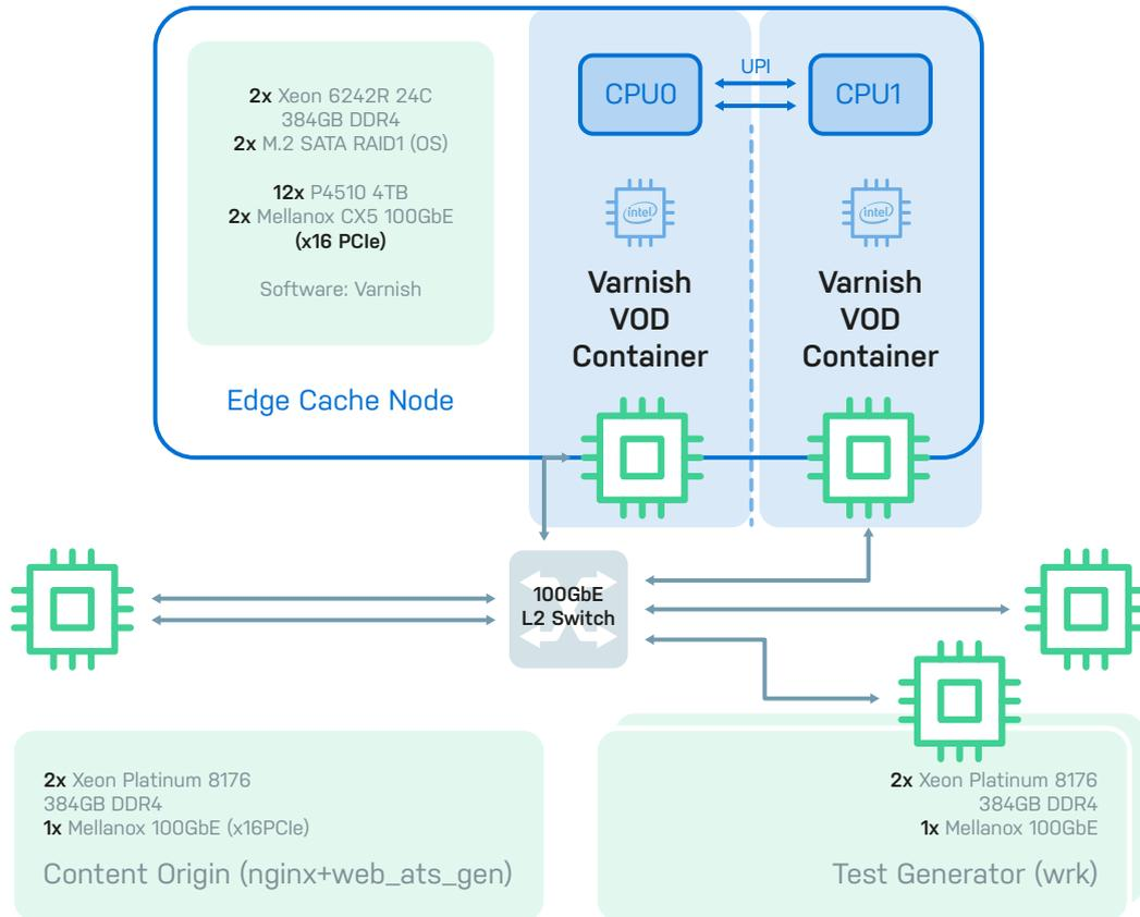
Figure 2: Containerized CDN test environment
