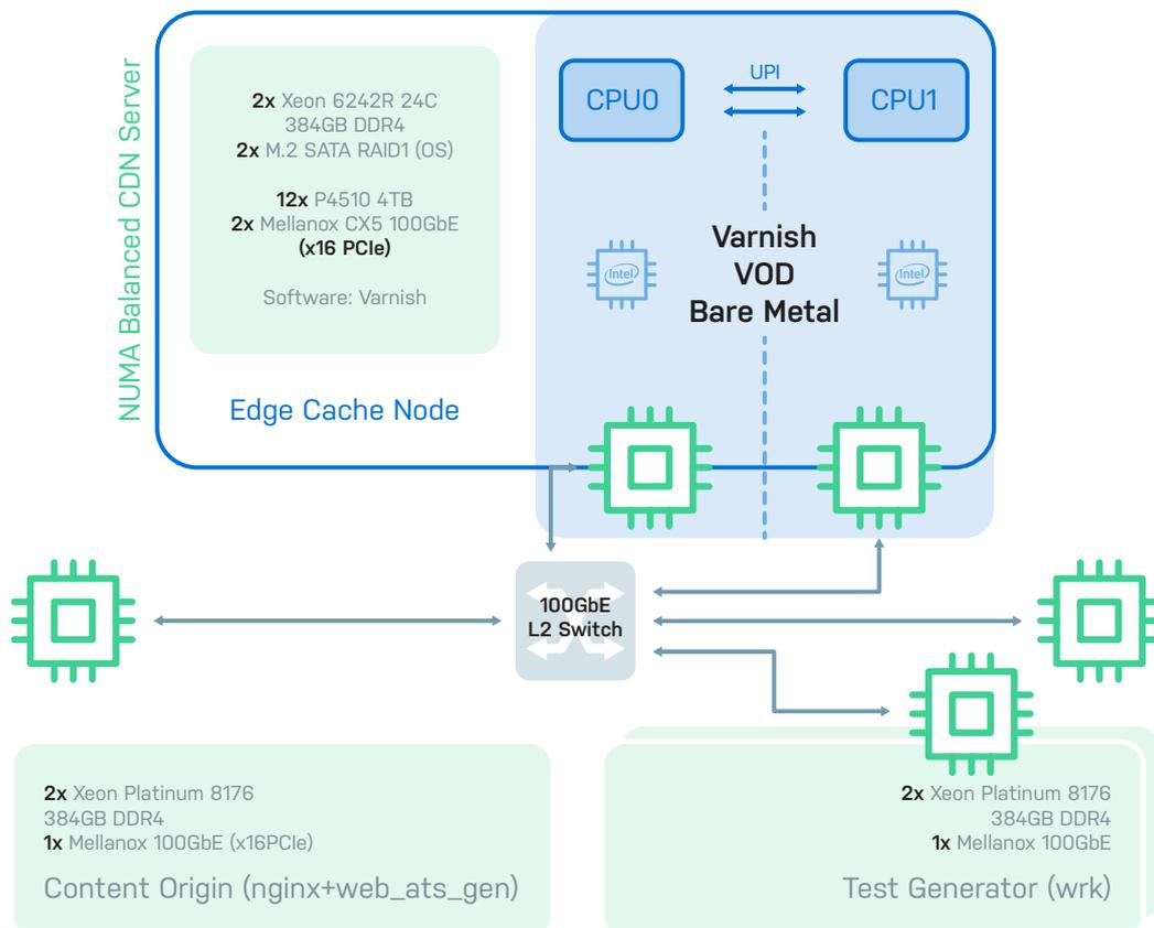
Figure 1: Bare metal CDN test environment
