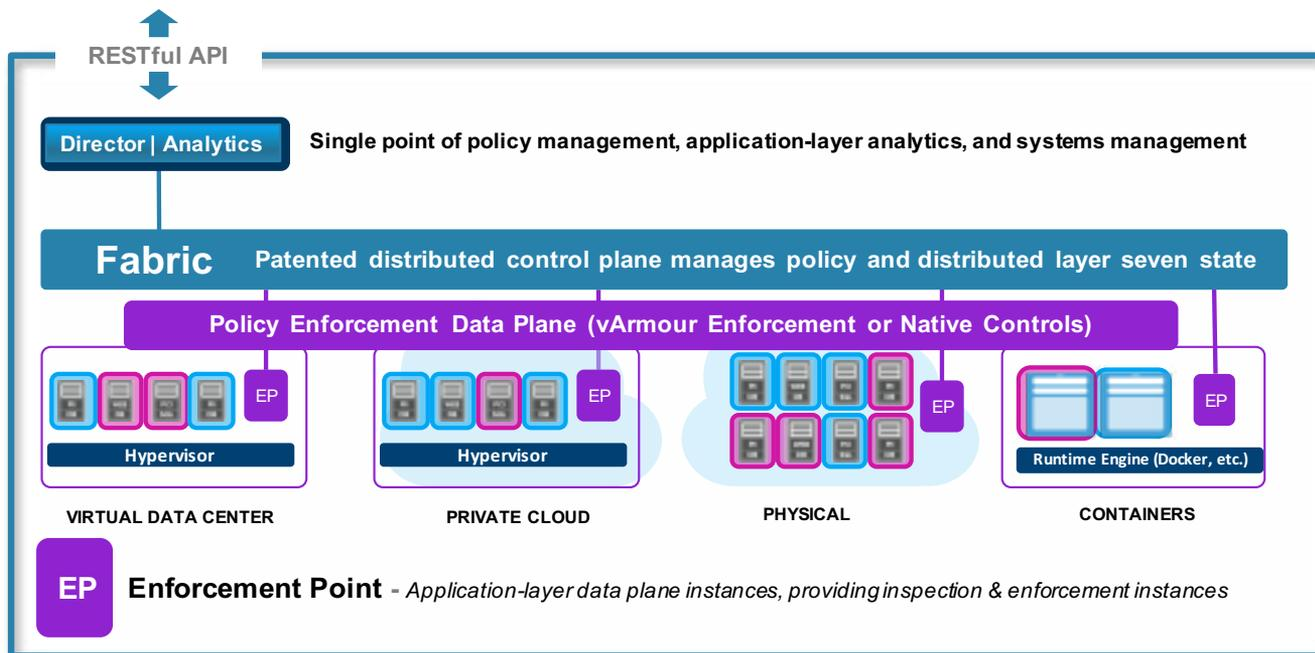
Figure 1. vArmour system architecture<sup>1</sup>
