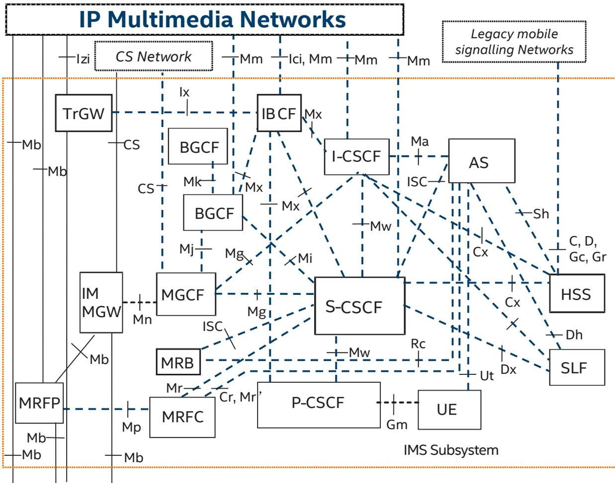
Figure 2. IMS reference architecture.
