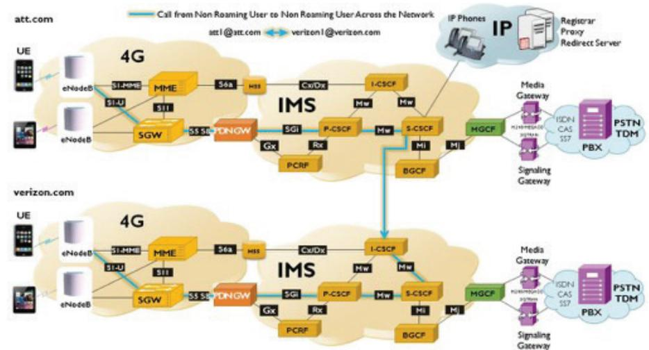
Figure 1. IMS control/signaling network overview.
