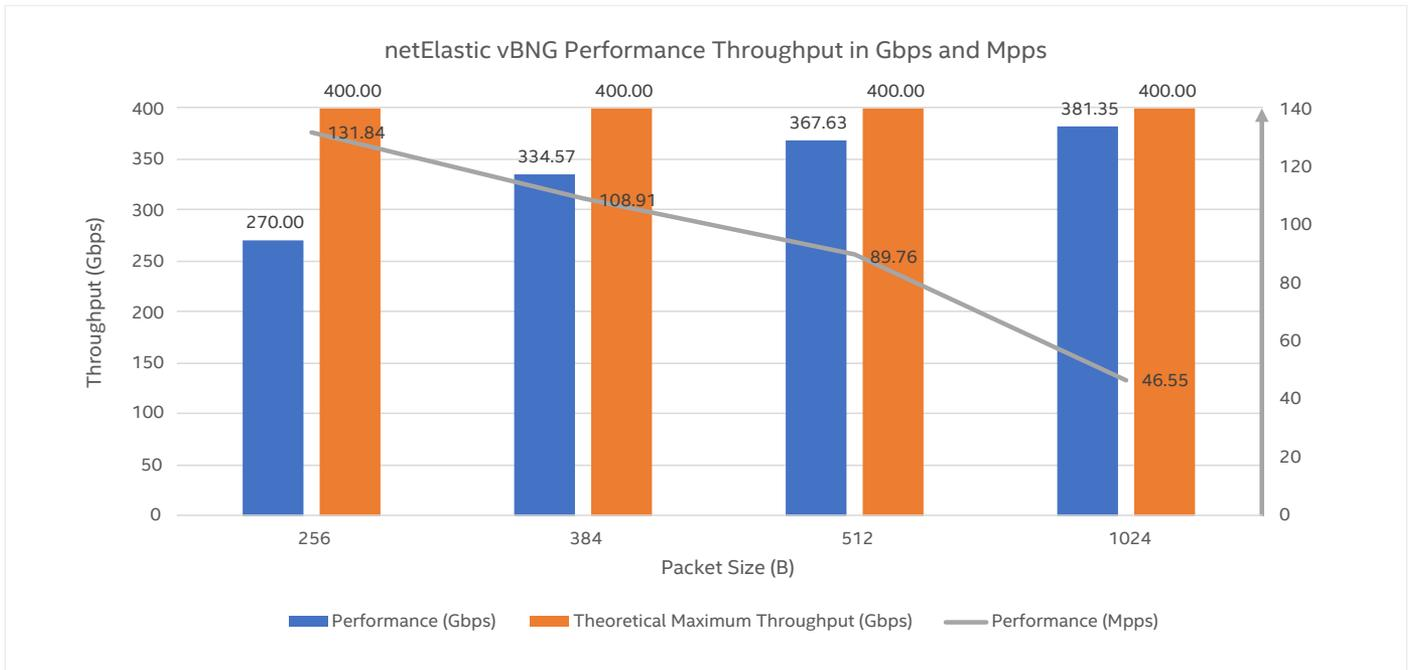
Figure 4. netElastic vBNG throughput in Gbps and Mpps (higher is better).<sup>1</sup>
