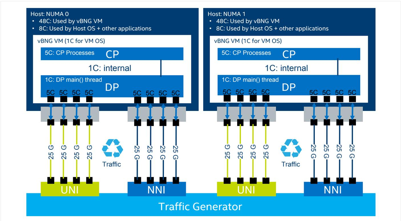
Figure 3. Test node block diagram
