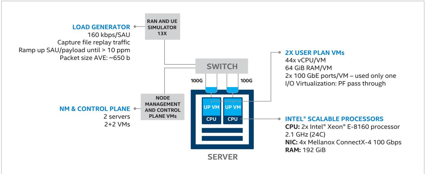
Figure 1. UP Testing Setup
