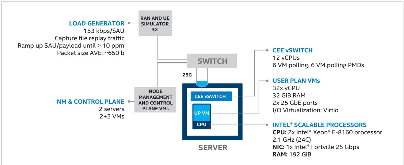
Figure 3. OVS Testing Configuration
