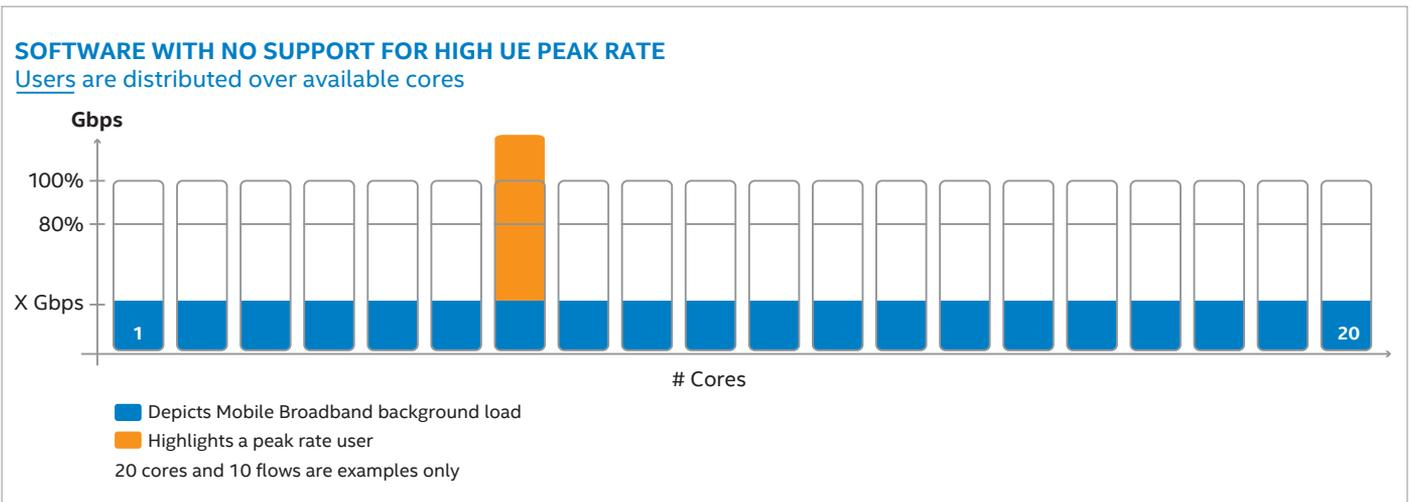
Figure 5. Inefficient Peak Rate Handling with Traditional UPF Implementation
