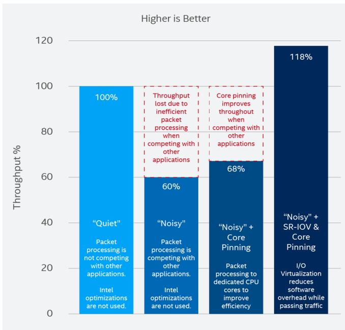
Figure 3. Impact of Intel optimizations on Throughput
