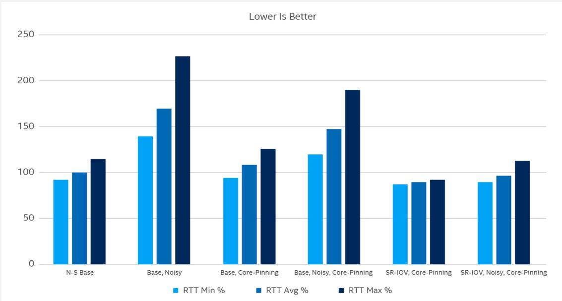
Figure 6. Minimum, mean, and maximum RTT across configurations
