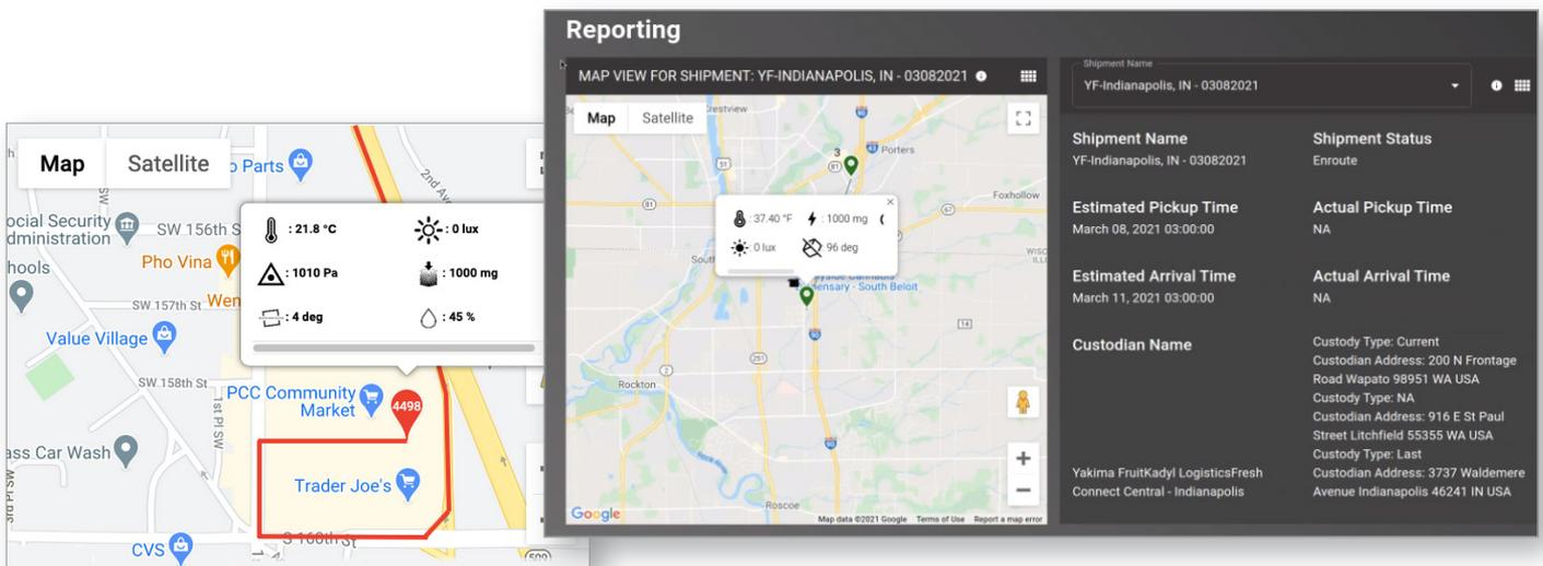
IoT sensors monitor the location, temperature, humidity, air pressure, light, shock, and tilt of perishable food packages or pallets in transit and communicate product status with supply chain partners via 5G and a shared ledger.
