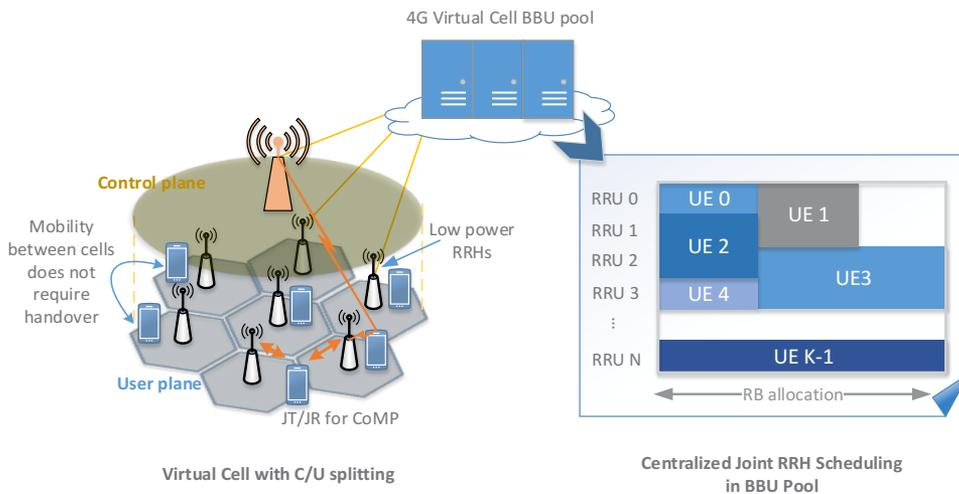
Figure 3. 4G Virtual Cell and joint scheduling in BBU pool
