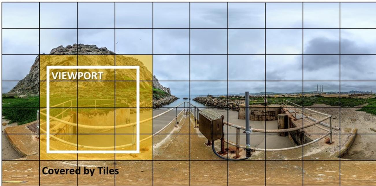
**Figure 1.** Image shows the viewport that is present on a VR device as a portion of the overall available image. Tiled streaming serves just the tiles needed for the viewport.<sup>1</sup>
