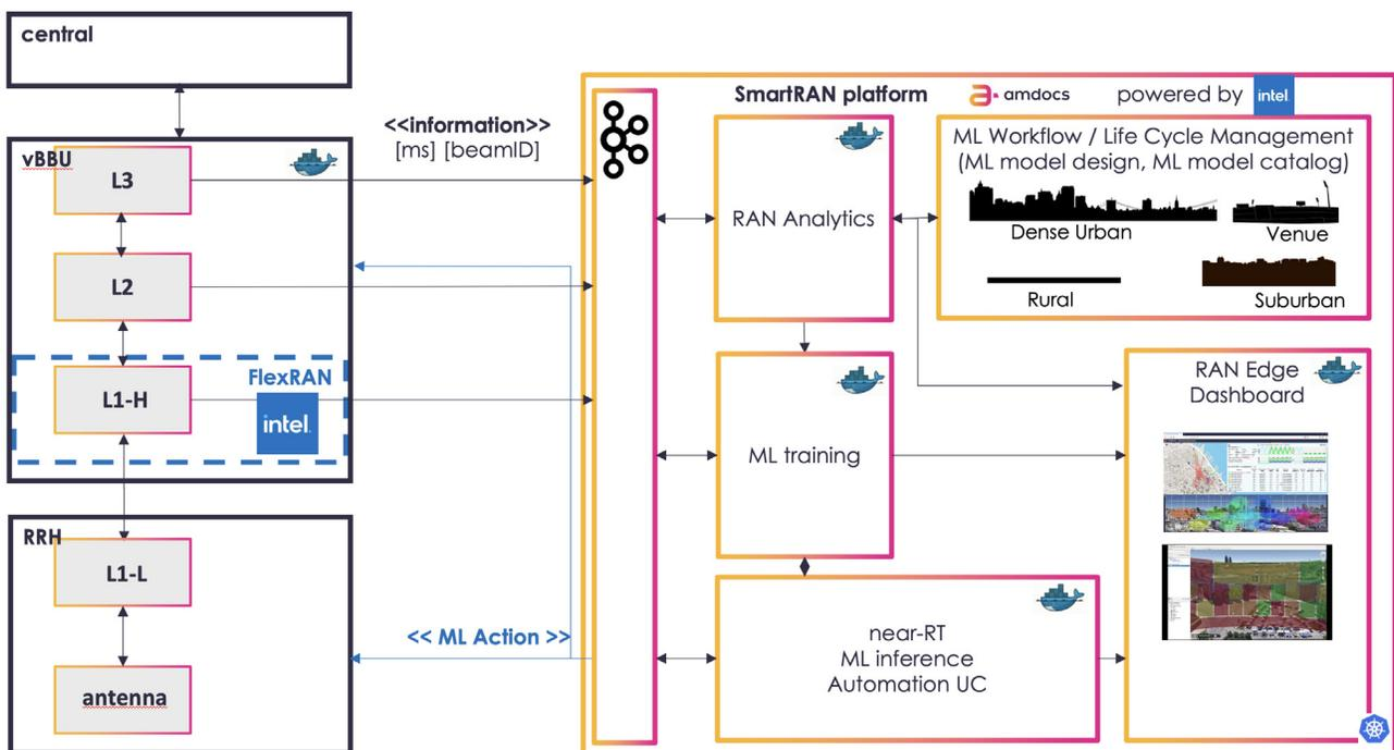
Figure 2. Amdocs SmartRAN solution architecture
