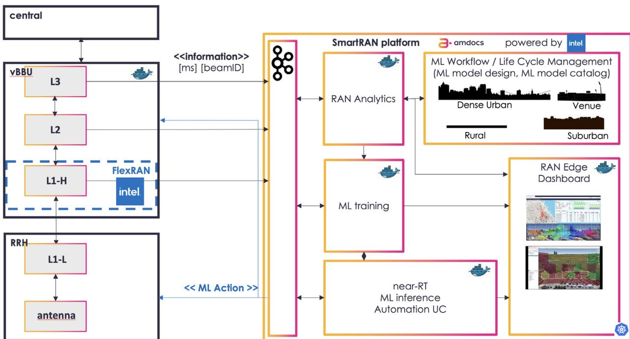
Figure 2. Amdocs SmartRAN solution architecture
