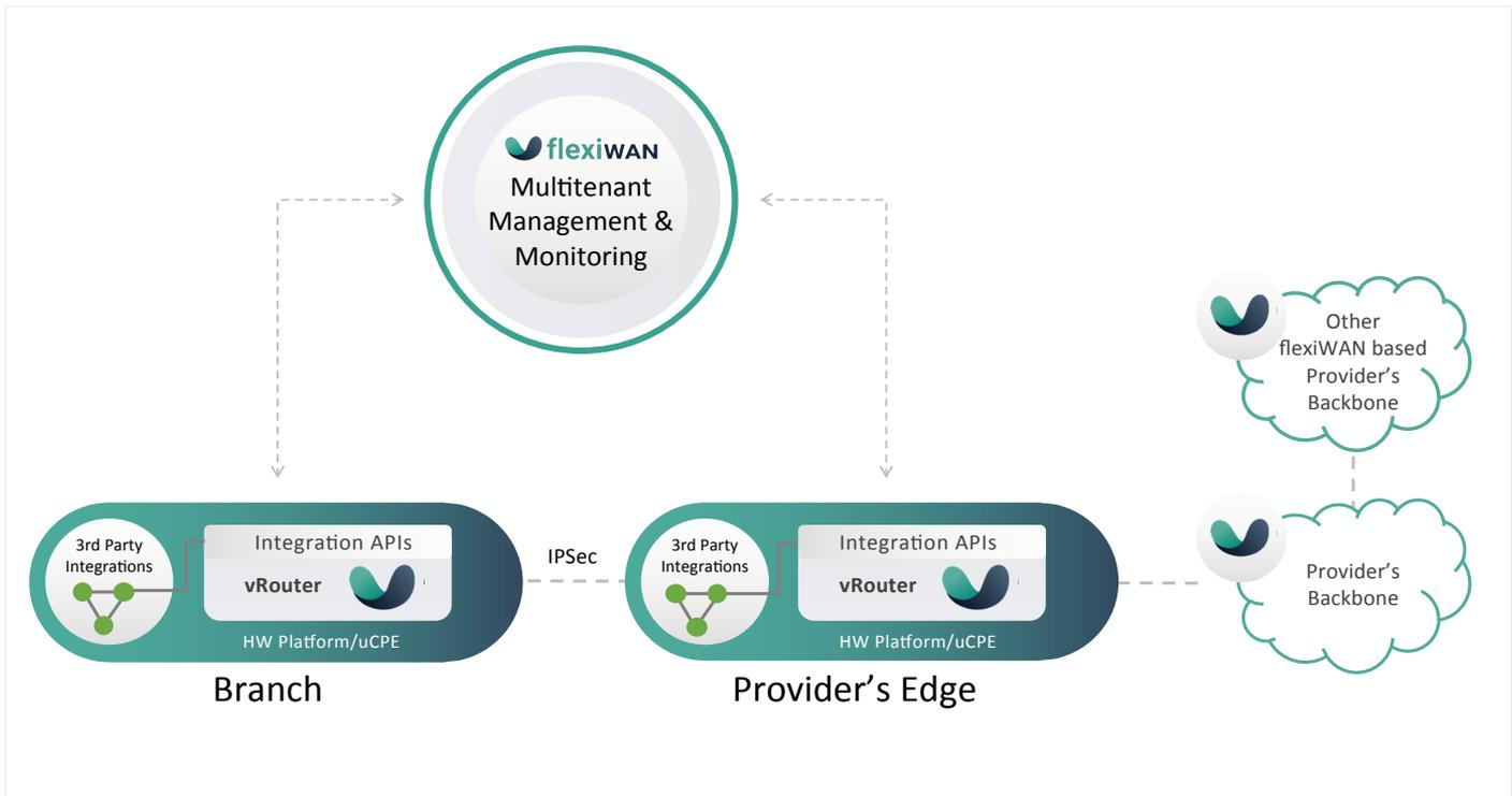
Figure 1. flexiWAN block diagram.<sup>2</sup>
