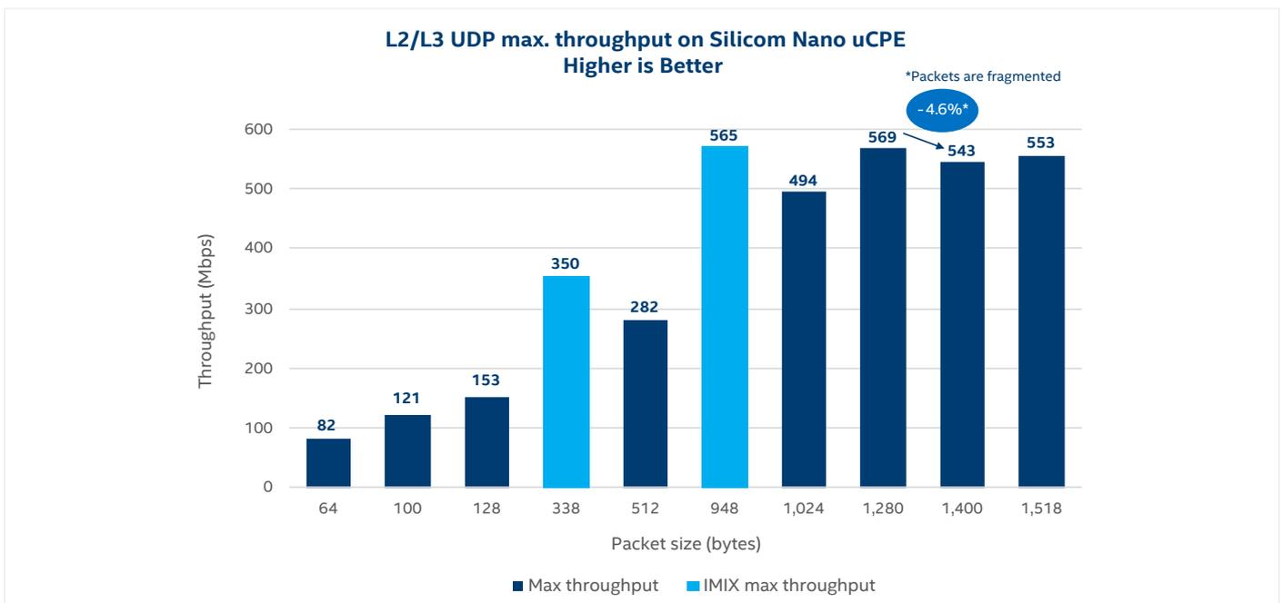
Figure 5. Layer 2/3 test results for Silicom Nano uCPE.<sup>1</sup>
