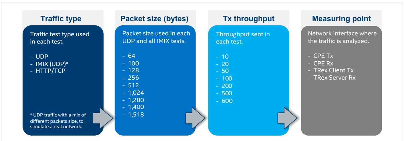
Figure 3. Test parameters.
