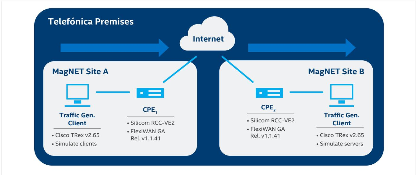
Figure 2. uCPE test configuration.
