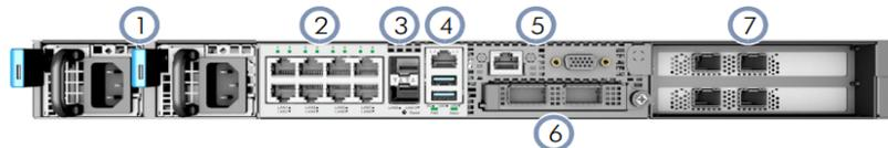
1. 2 x AC PSUs System LEDs
