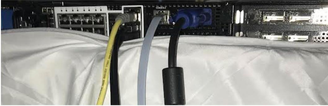
Figure 2 Patch Cable Connected to Console RJ45
