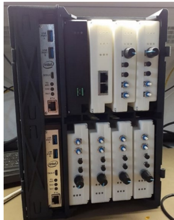
Figure 4: Intel E4S prototype hardware rendering and photo of a fully populated test system. A mechanical restraint on the left partially covers the two compute modules. The power module is in black color, and the remaining modules in white. The switch module is in the center position at the top. All six of the input/output modules shown are for testing and have knobs, buttons, and LED indicators used for thermal and interface testing.
