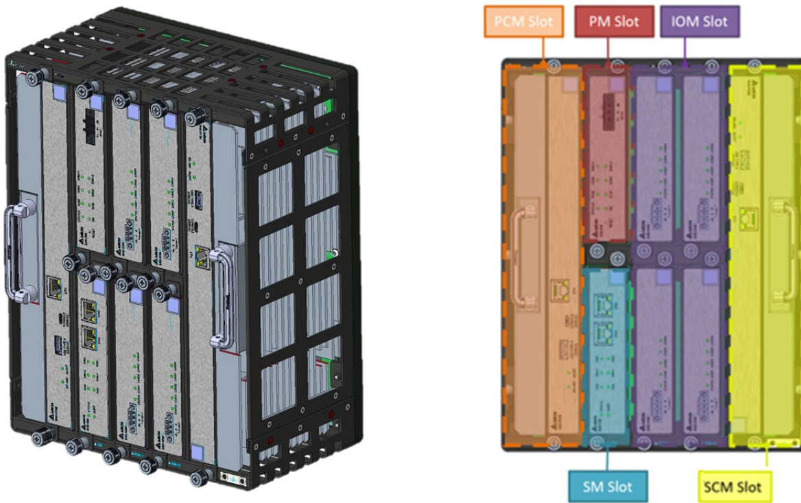
Figure 6: Industrialized mechanical design for the field tests. The compute modules are located at the left and right sides. There are the power module, switch module, and four IO modules. The outer housing is opened in strategic locations to optimize airflow and passive cooling.
