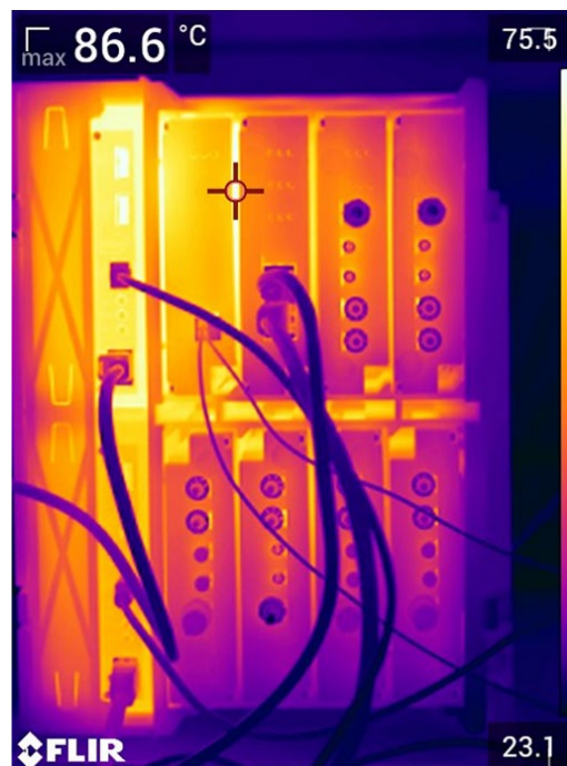
Figure 5: Thermal simulation (left) in an enclosed plastic cabinet box with additional hardware – qualitative results show the relative temperature distribution. On the right is an image of the real prototype provided by a FLIR thermal imaging camera. The system is under full load in an open lab environment.
