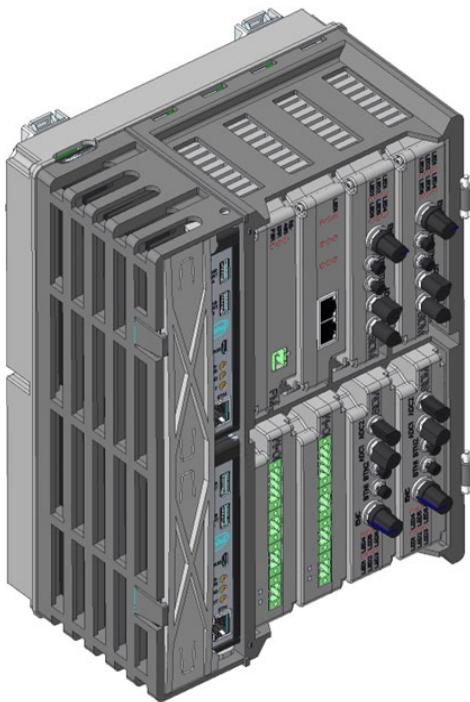
Figure 4: Intel E4S prototype hardware rendering and photo of a fully populated test system. A mechanical restraint on the left partially covers the two compute modules. The power module is in black color, and the remaining modules in white. The switch module is in the center position at the top. All six of the input/output modules shown are for testing and have knobs, buttons, and LED indicators used for thermal and interface testing.
