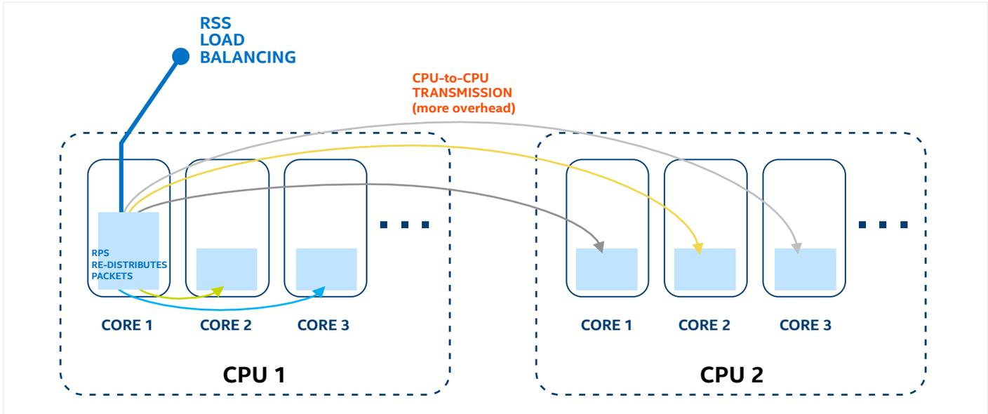
Figure 6. The packet distribution with RPS
