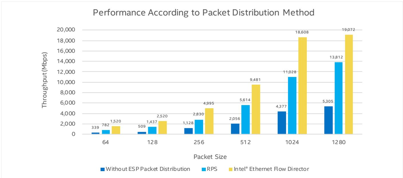
**Figure 11.** Performance according to packet distribution method<sup>1</sup>
