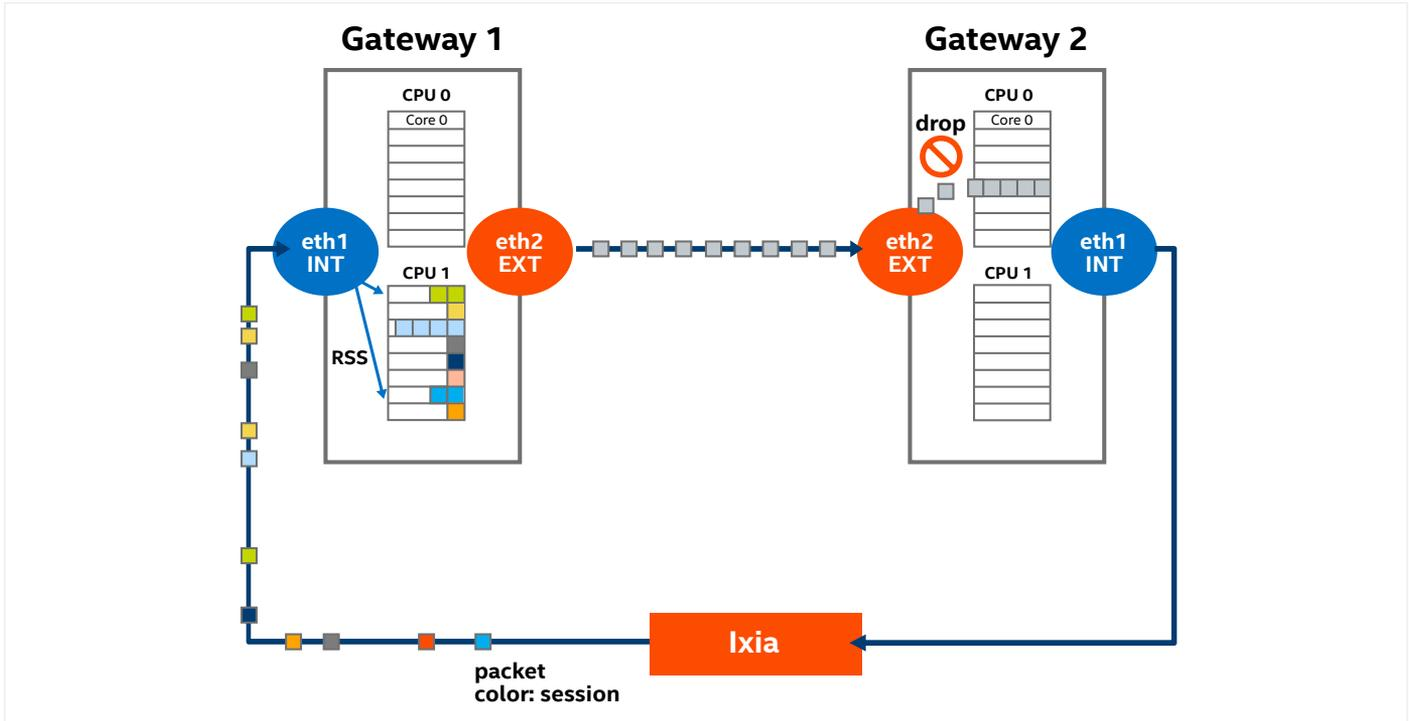
Figure 2. The flow and distribution of packets in IPsec VPN
