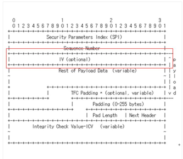
Figure 4. The packet architecture<sup>2</sup>
