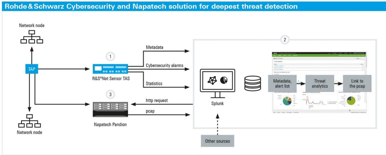
**Figure 1.** R&S Net Sensor capturing and processing data packets<sup>1</sup>
