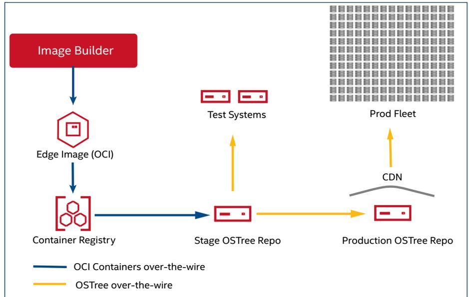
Figure 4. Image Builder operations from image to target
