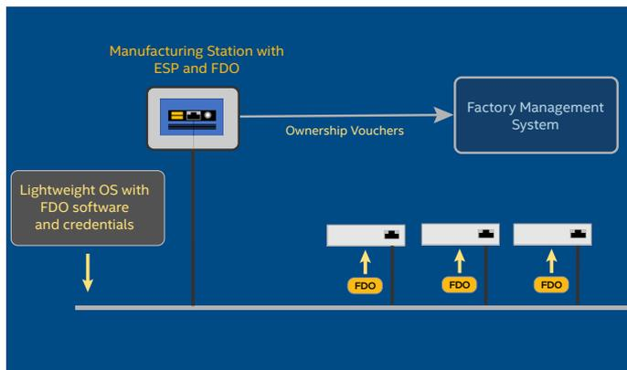
Figure 2. ESP Manufacturing environment to initialize FDO with a lightweight OS
