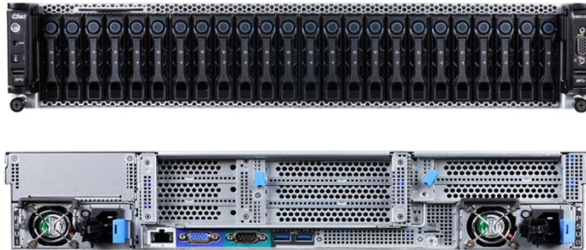
Figure 2: Front and rear views of QuantaGrid D52BQ-2U
