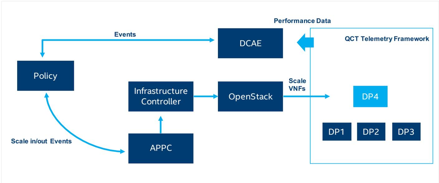
Figure 6. Auto-scaling closed loop automation—run time.
