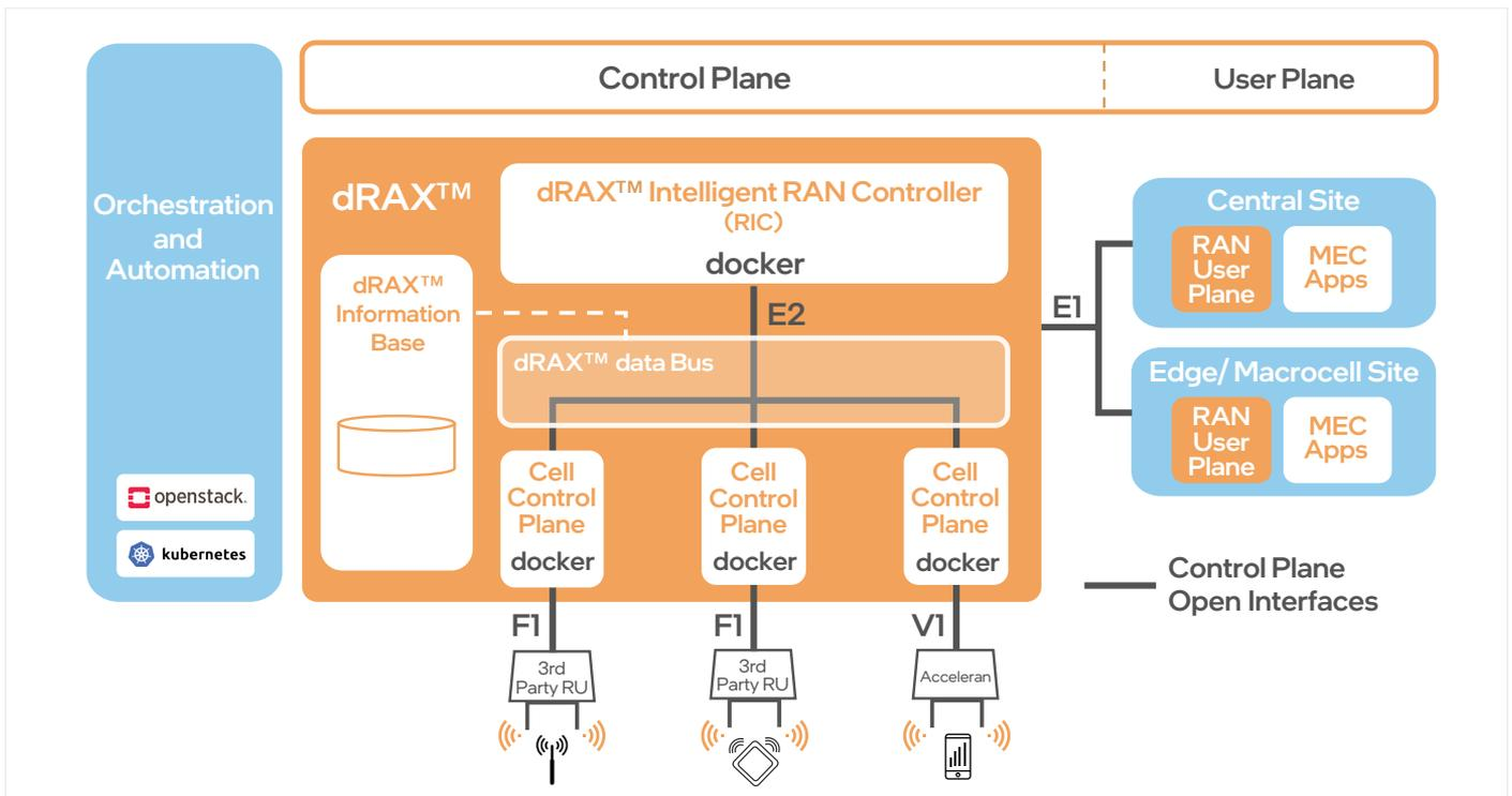
Figure 2. Accelleran dRAX block diagram.
