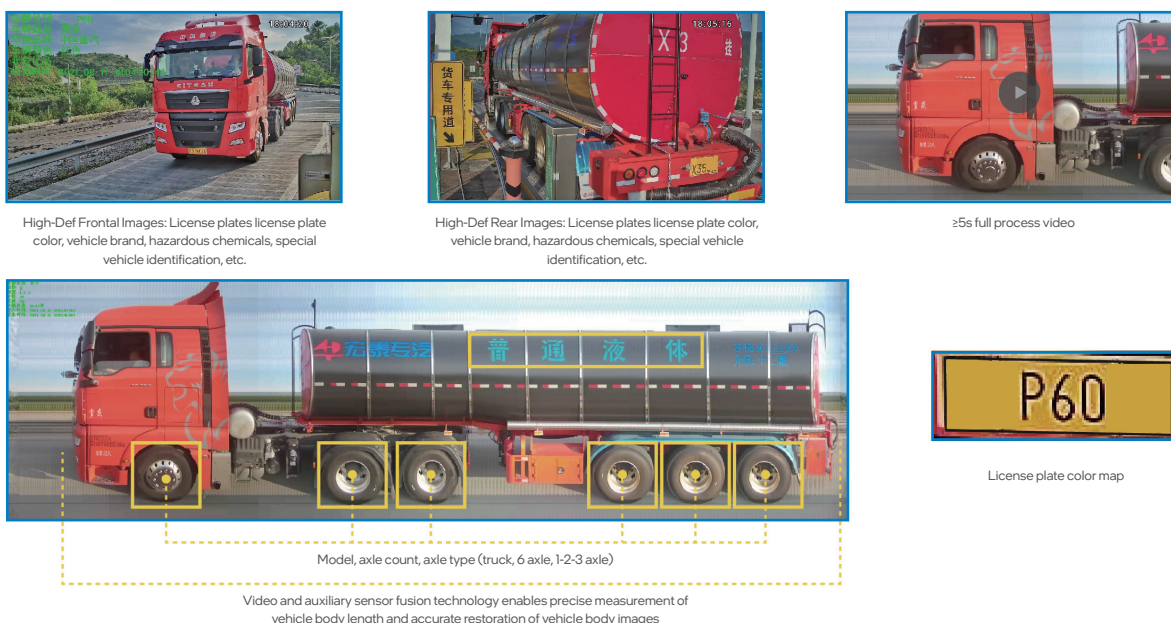
Figure 2. Vehicle Feature Extraction Performed by the Xiaoshen Hitomi Toll Vehicle Identification and Management Solution
