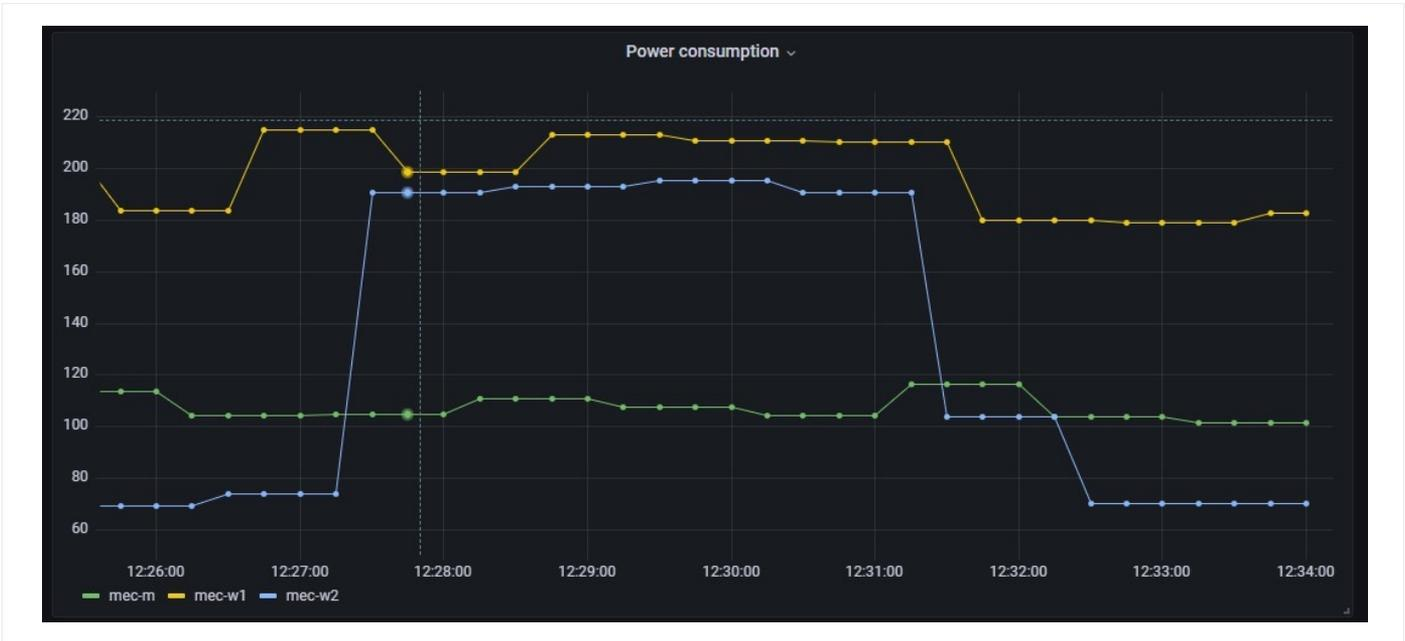
Figure 14. Power Consumption of the Node (mec-w2) when it is scaled-in and scaled-out
