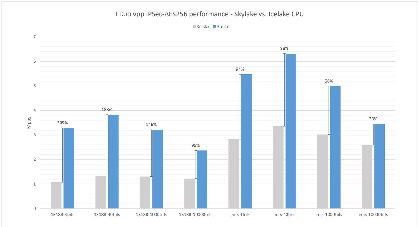
Figure 2. FD.io CSIT - IPsec packet forwarding performance.
