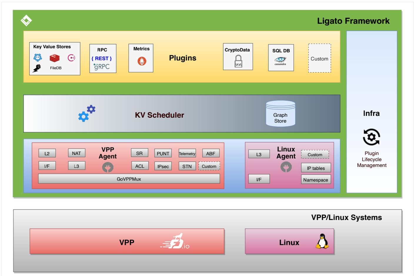
Figure 1. Ligato block diagram.
