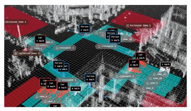
Solutions that integrate <u>LiDAR</u> with edge processing, like the one developed by Outsight, are making this a reality. By deploying this technology at intersections, cities can gather the data needed to prevent accidents before they happen, moving from reactive analysis to proactive prevention.
