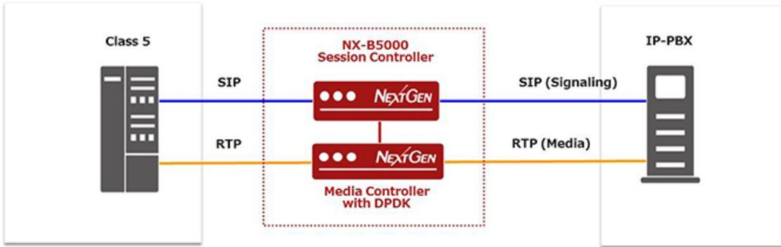
Figure 1. Architecture of the NX-B5000 showing the role of the Session Controller and Media Controller<sup>2</sup>
