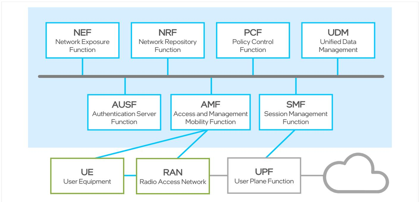
Figure 1. Core components of 5G virtual core.
