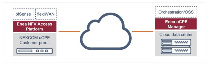
**Figure 3.** Block diagram of demonstration setup including Enea NFV Access Platform as the provider of all network functions virtualization infrastructure (NFVI)
