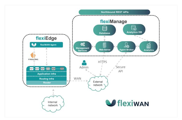
Figure 4. flexiWAN SD-WAN architecture, including the flexiEdge and flexiManage software
