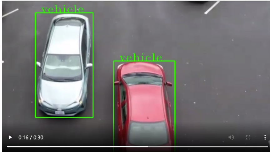
Figure 3: Edge AI Box test results with rectangle bounding boxes and object labels over the videos
