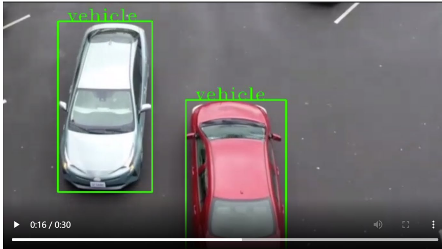
Figure 3: Edge AI Box test results with rectangle bounding boxes and object labels over the videos
