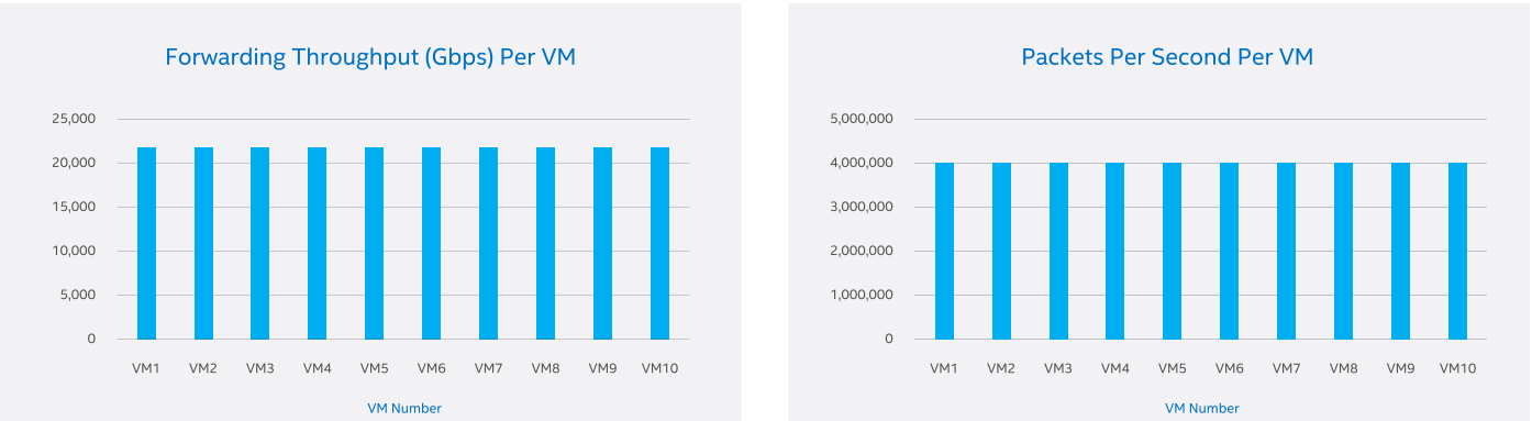
Figure 11: Dual Intel® Xeon® Gold 6230 Processor Performance: Forwarding Throughput and Packets per Second per Virtual Machine (VM)
