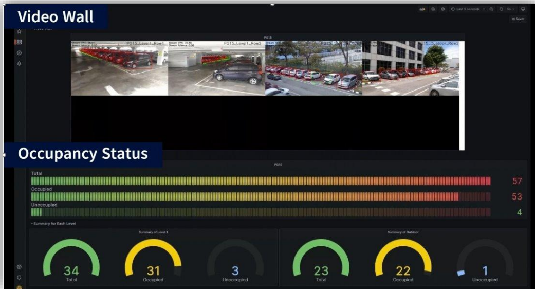
Real-time parking space detection and occupancy monitoring
