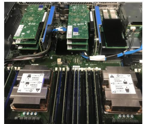
Figure 9. UPF Server (2x6252N with Intel® Network Adapters)
