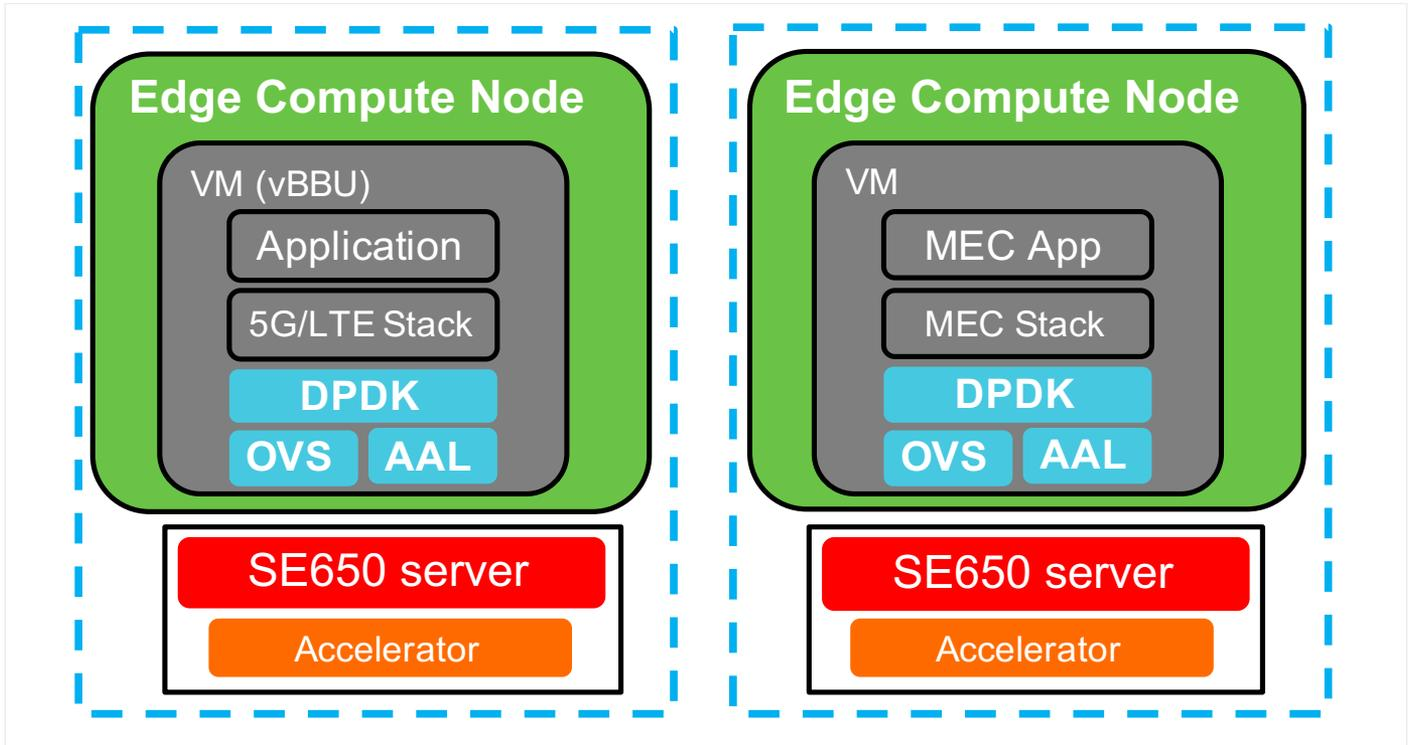
Figure 2. Block diagram to the left is an example stack for a 5G application and on the right is the MEC software stack
