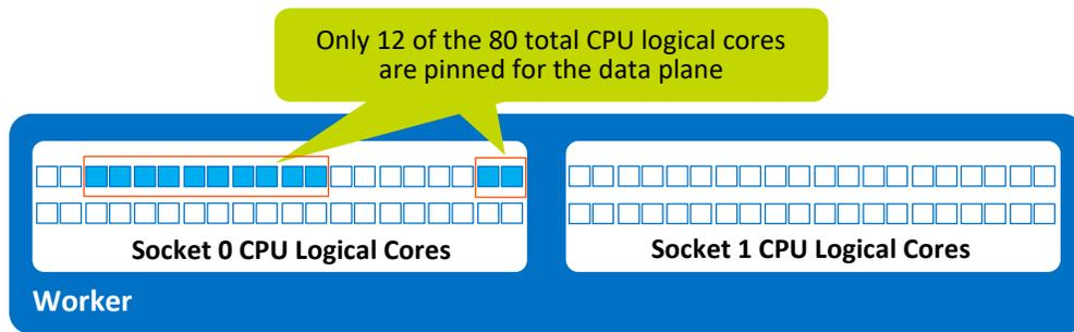
Figure 5. Server CPU Logical Core Allocation for 5G Data Plane
