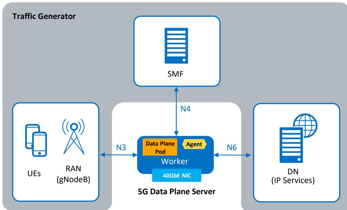
Figure 3. Data Plane Server in an Emulation Environment
