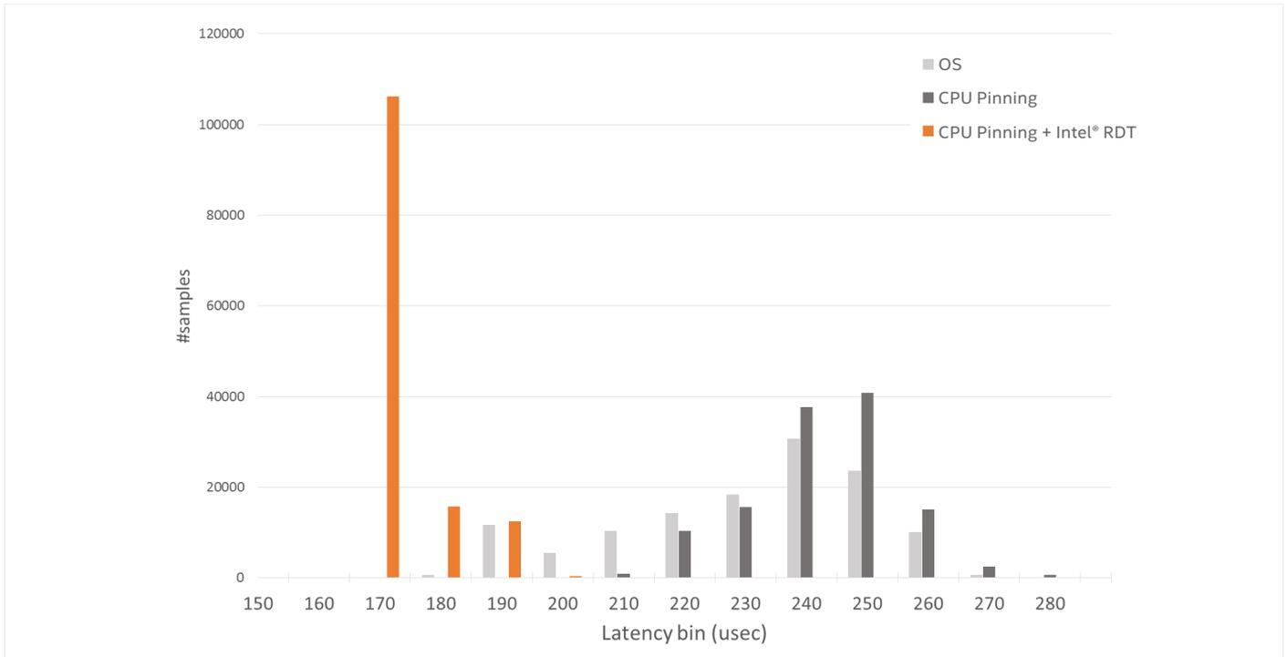
**Figure 1. vRouter performance measured in microseconds (µs) under three test scenarios.<sup>2</sup>**
