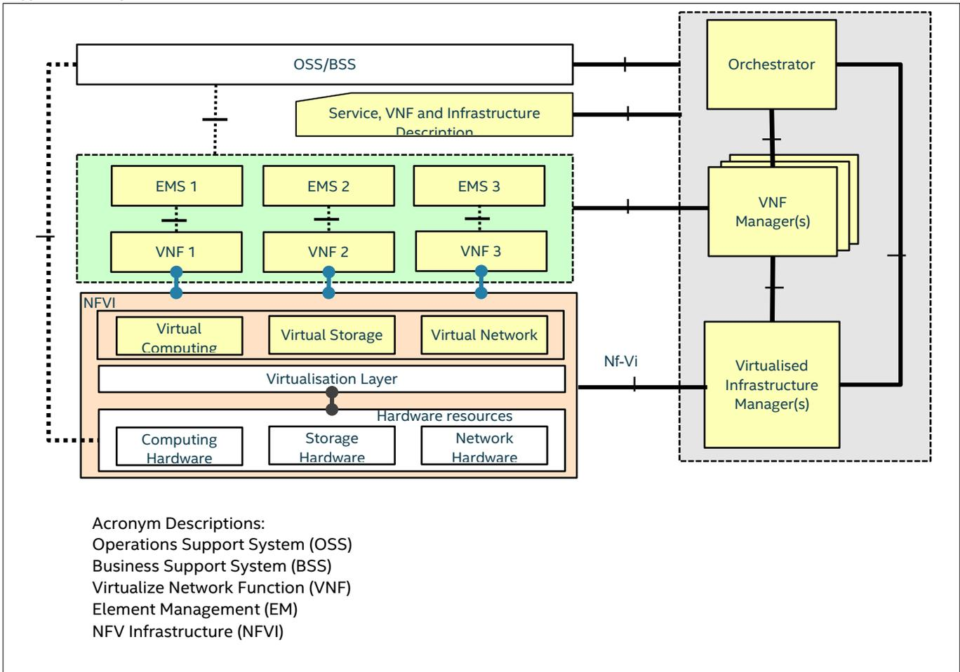
An simplify NFV test environment used by this document specified by the diagram below:-
