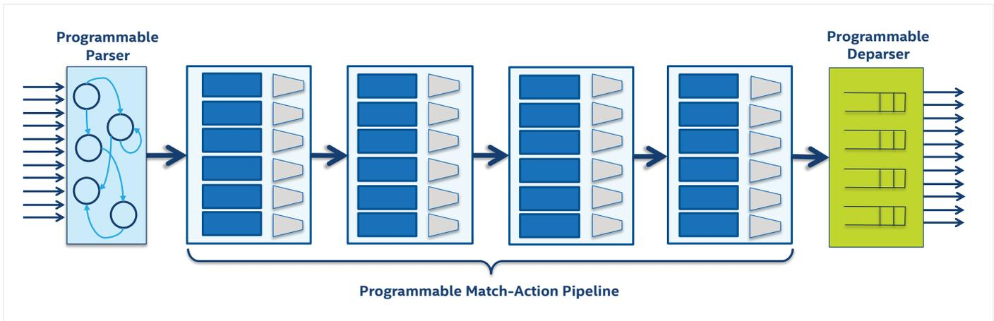
Figure 1. Match action engine in a P4 target.
