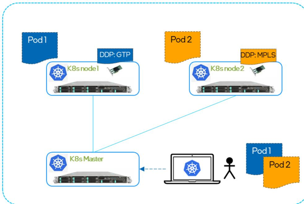
Figure 2. Workloads Deployment in K8s Cluster with SR-IOV Networking and DDP Package Request
