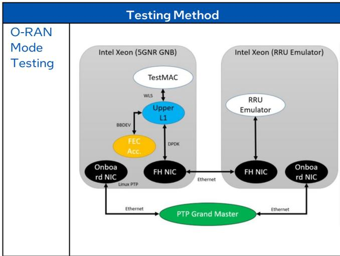
Table 6 shows the testing methods supported by the Intel FlexRAN™ reference software, timer mode and O-RAN mode.
