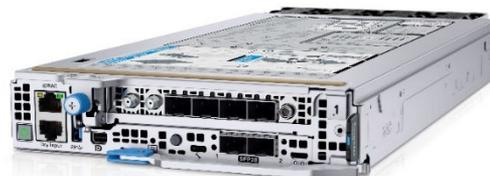
The 2U Compute Sled builds upon the foundation of the 1U Sled and adds support for an additional two x16 FHHL slots.
