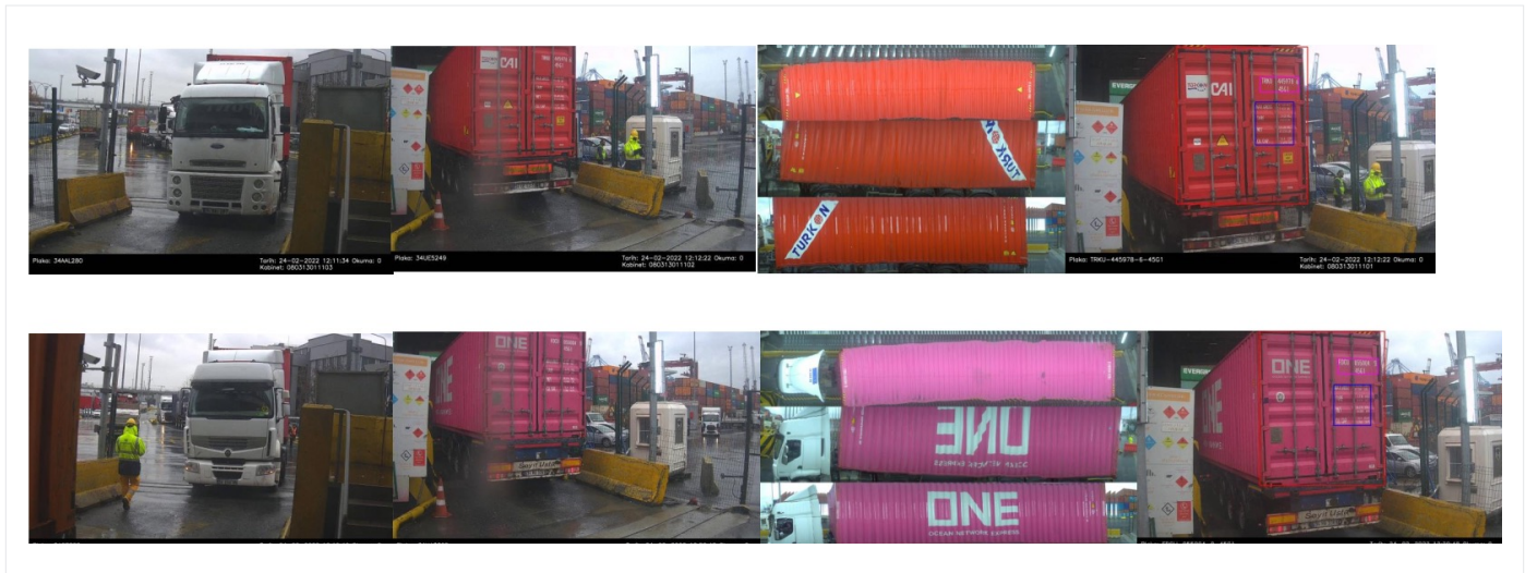
Figure 1. The ConScan container and truck identification recognition and tracking system output.
