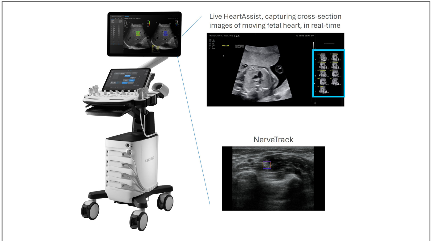
Figure 1. Samsung Medison V4 ultrasound is one model that targets use of Intel Core Ultra processors for AI capabilities. Call outs show examples of imaging from Live HeartAssist and NerveTrack.
