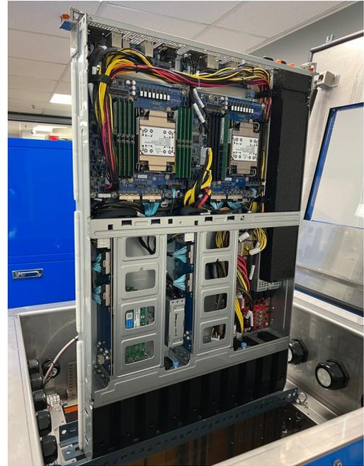
**Figure 4.** Intel 2U modular server chassis
