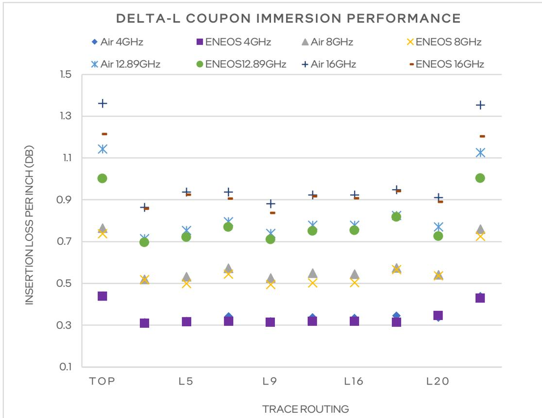
Figure 7. Insertion loss comparison
