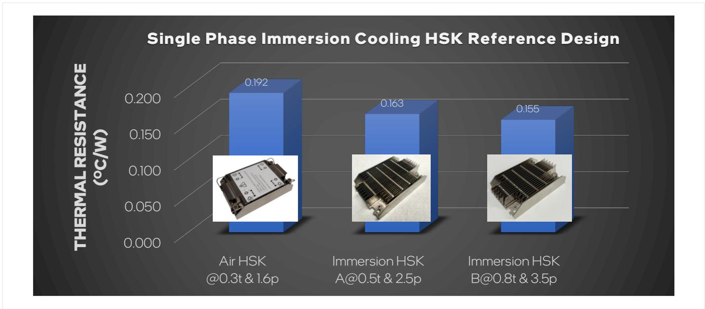
Figure 10. The results of heat sink verification
