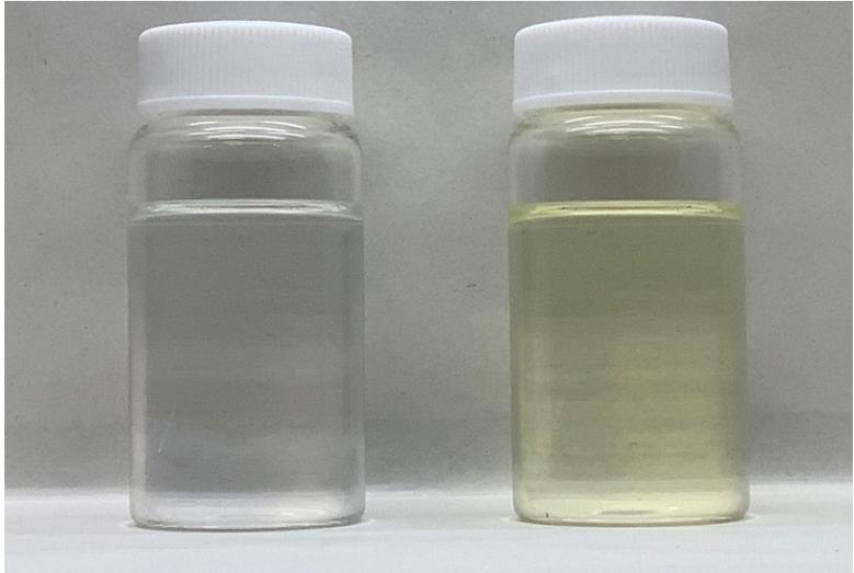
**Figure 11.** New ENEOS immersion cooling fluid (left) and general lubricant base oil (right)
