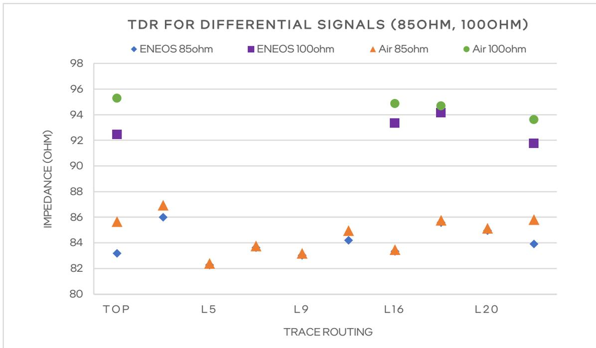
A. TDR test for differential signals
