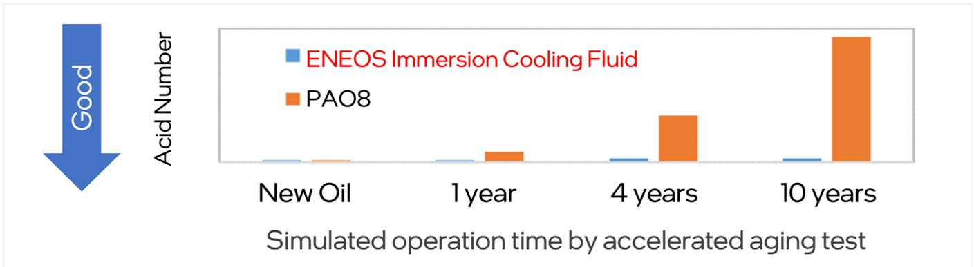
**Figure 12.** ENEOS immersion cooling fluid acceleration test result. Blue indicates ENEOS immersion cooling fluid and orange is general lubricant (lower is better)
