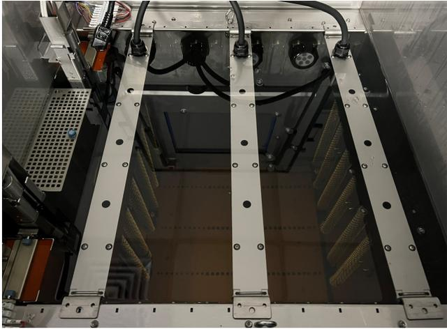
**Figure 3.** Three sets of dummy heaters are placed in the experimental equipment
