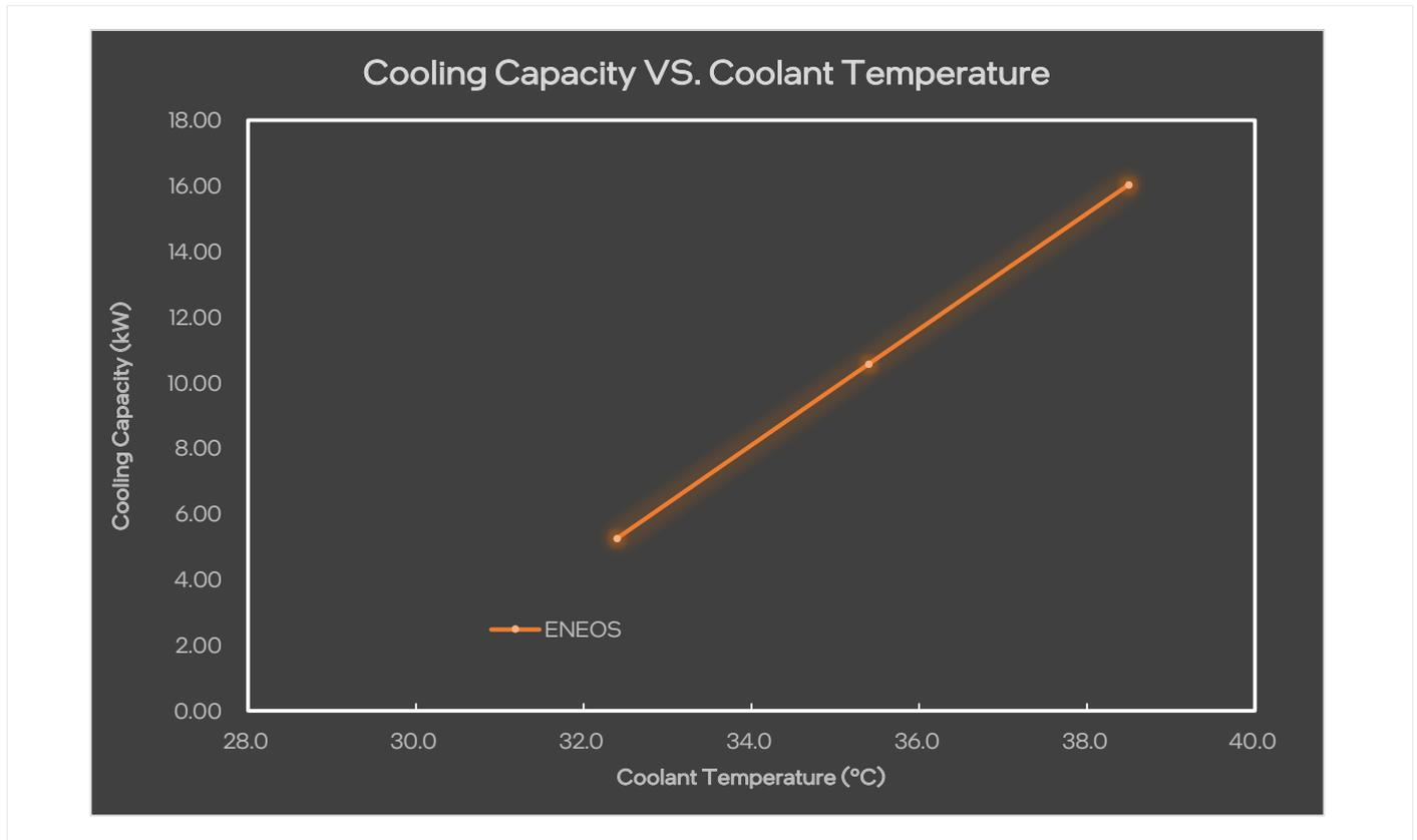
Figure 5. Cooling capacity and coolant inlet temperature test results
