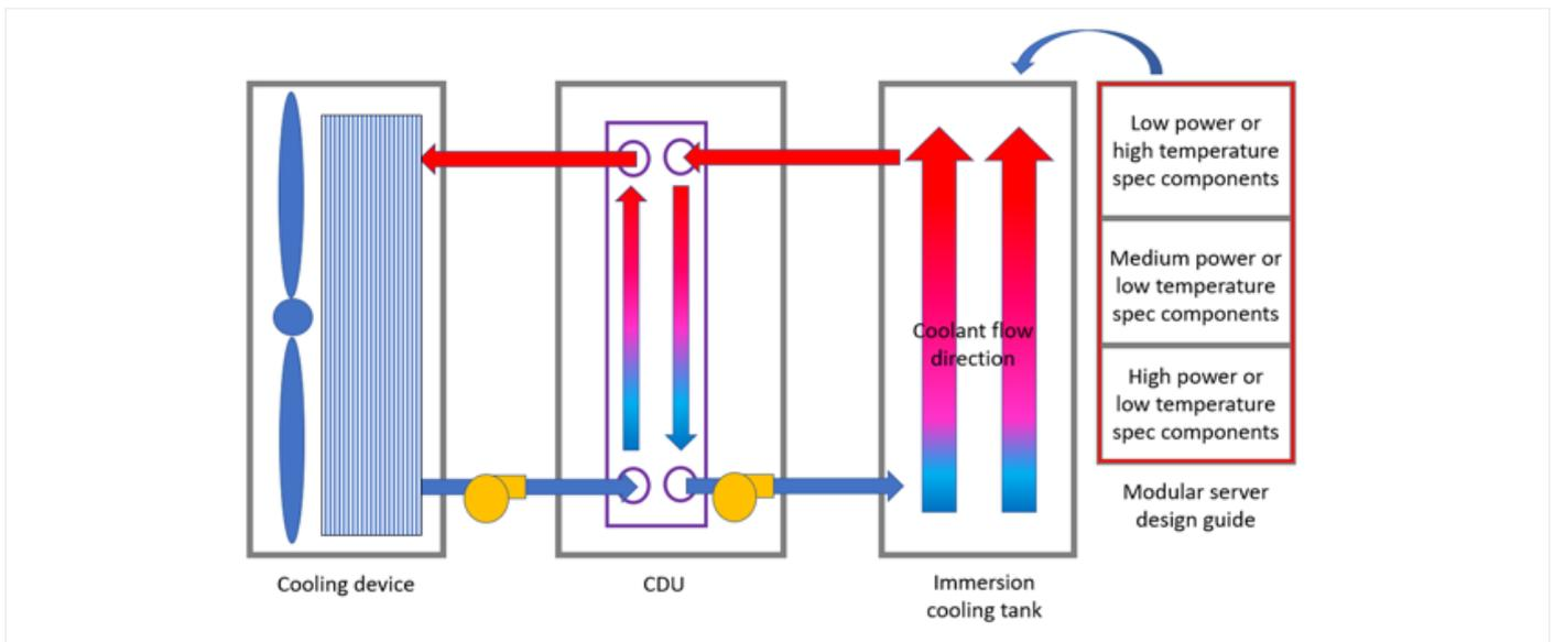
Figure 1. Single phase immersion cooling working principle with modular server design guide
