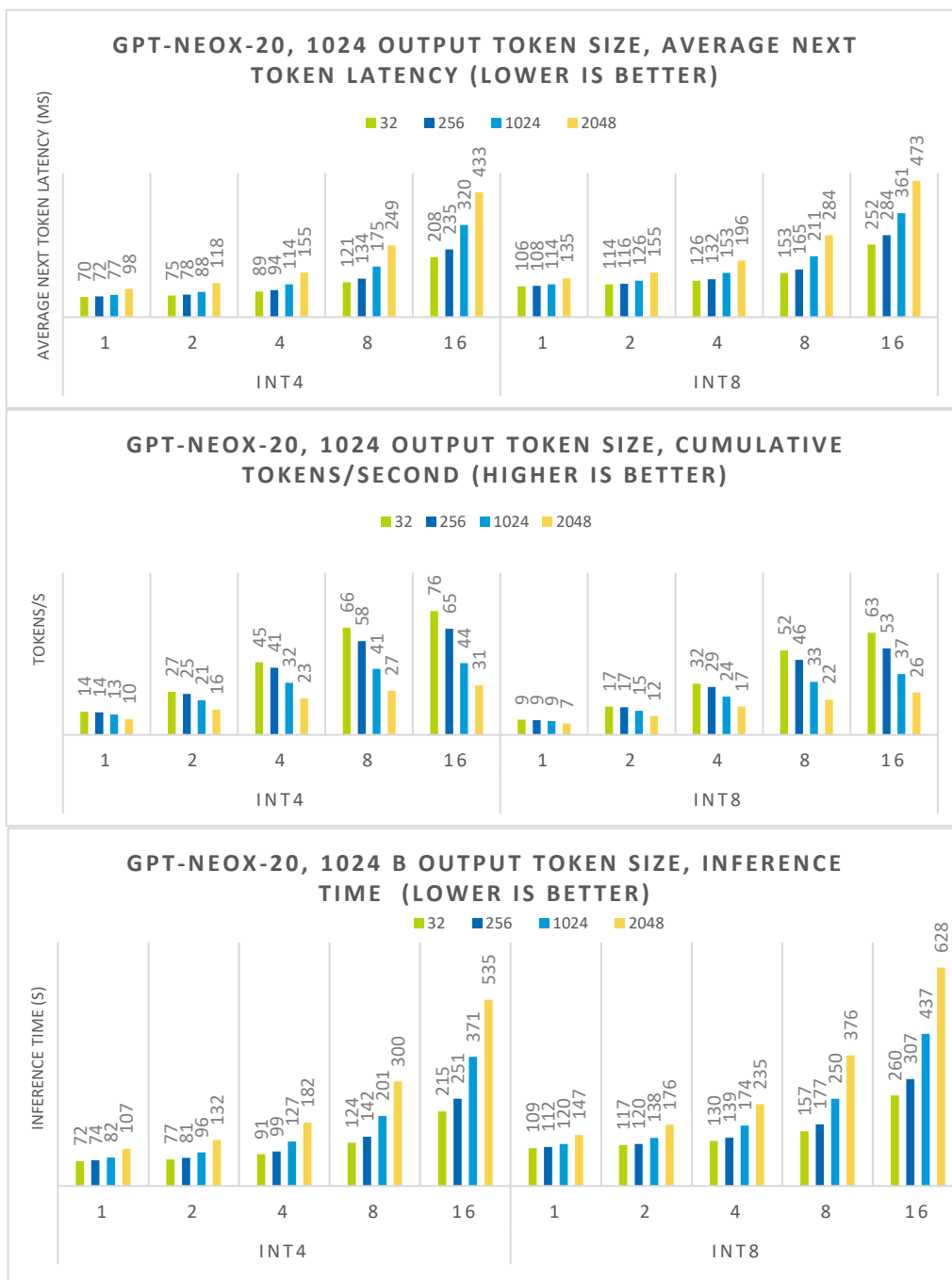
Figure 9 Performance for GPT-NEOX 20B Model on Supermicro E403 (CPU only)
