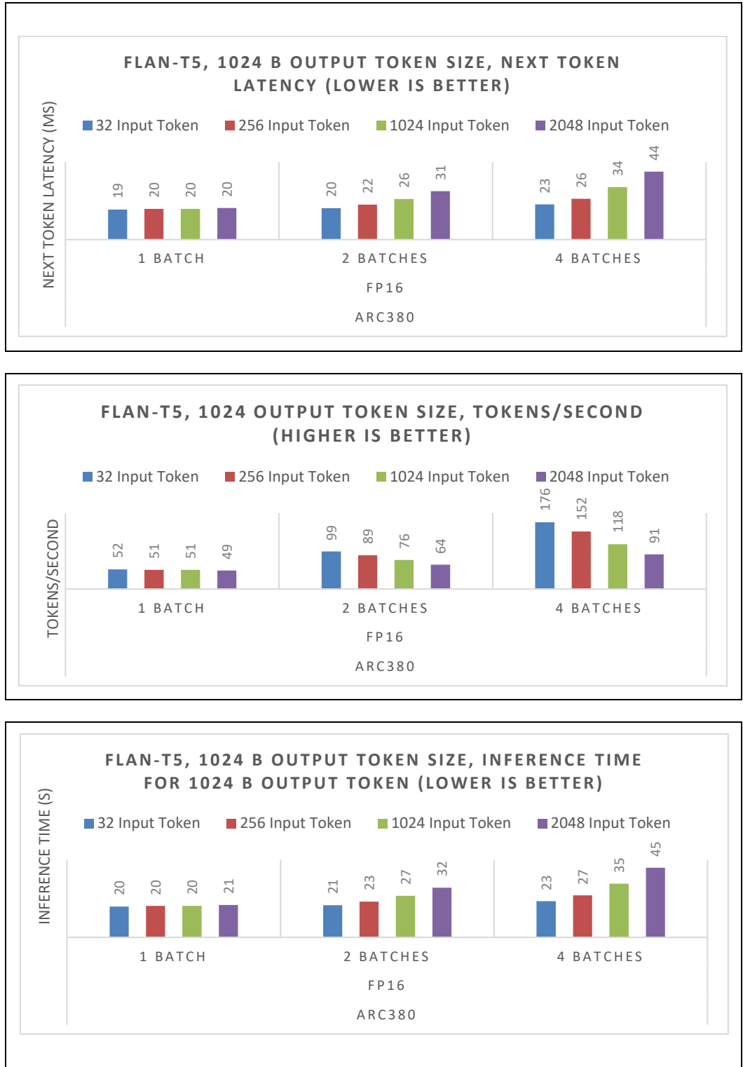
Figure 8. Gen AI Entry Configuration Performance Graph (flan-t5 with Intel® ARC380)
