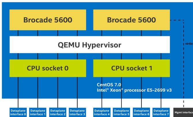
Figure 17. High level architecture: two instance, each on its own CPU socket
