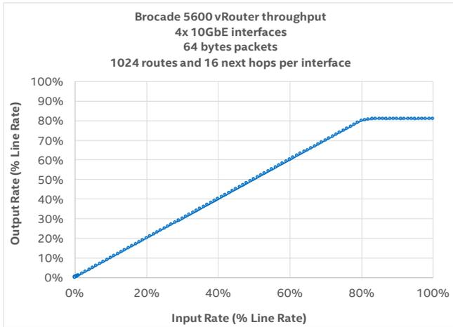
Figure 6. Brocade 5600 vRouter throughput<sup>7</sup>
