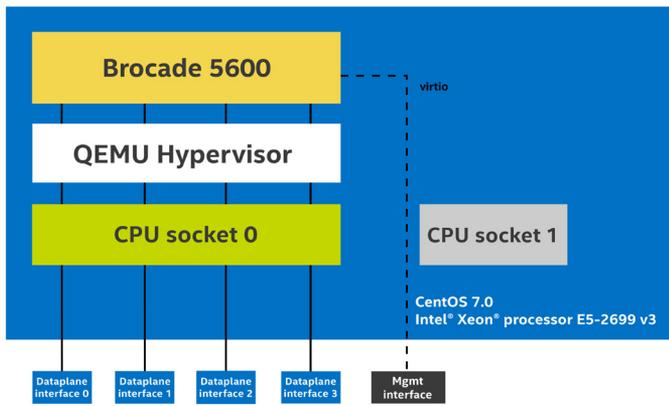
Figure 16. High level architecture – one instance on one socket
