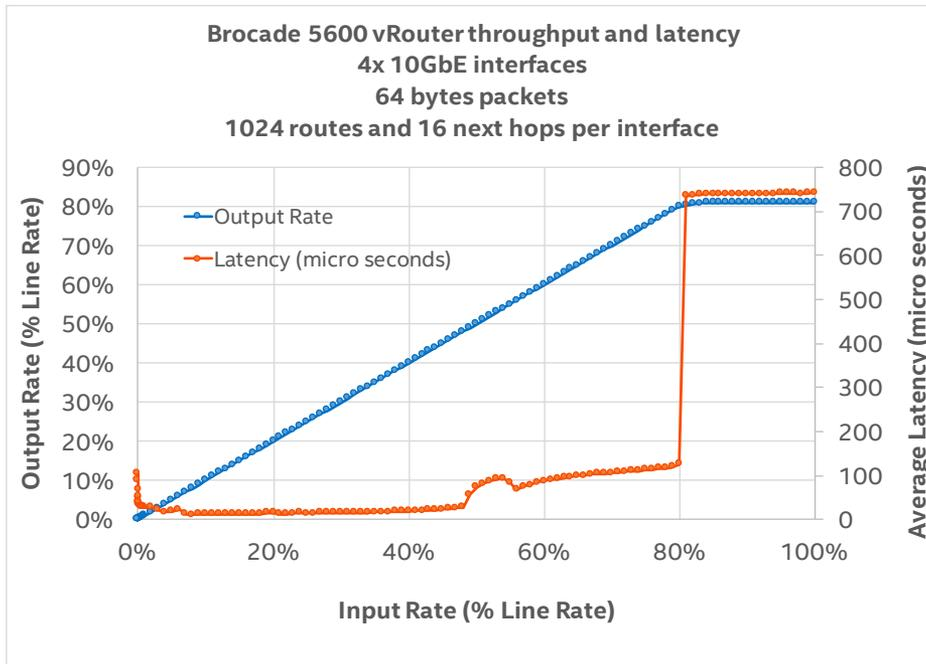
Figure 2. vRouter's latency and throughput in function of the input rate<sup>1</sup>
