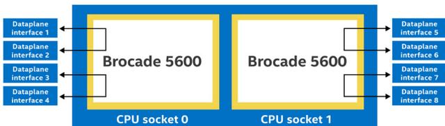
Figure 13. Two instance of vRouters, each on its own CPU socket
