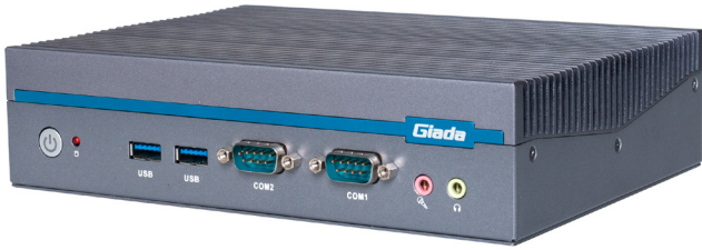
Figure 1. The front-panel of the Giada AE613 features two USB 3.2 Gen 2 ports, two COM ports, and audio out and microphone in jacks. Ports on the back panel include two HDMI connectors, one DisplayPort, two 1GbE LAN connections, two more USB 3.2 ports and two USB 2.0 ports. The system can accommodate two 4G cellular antennas.
